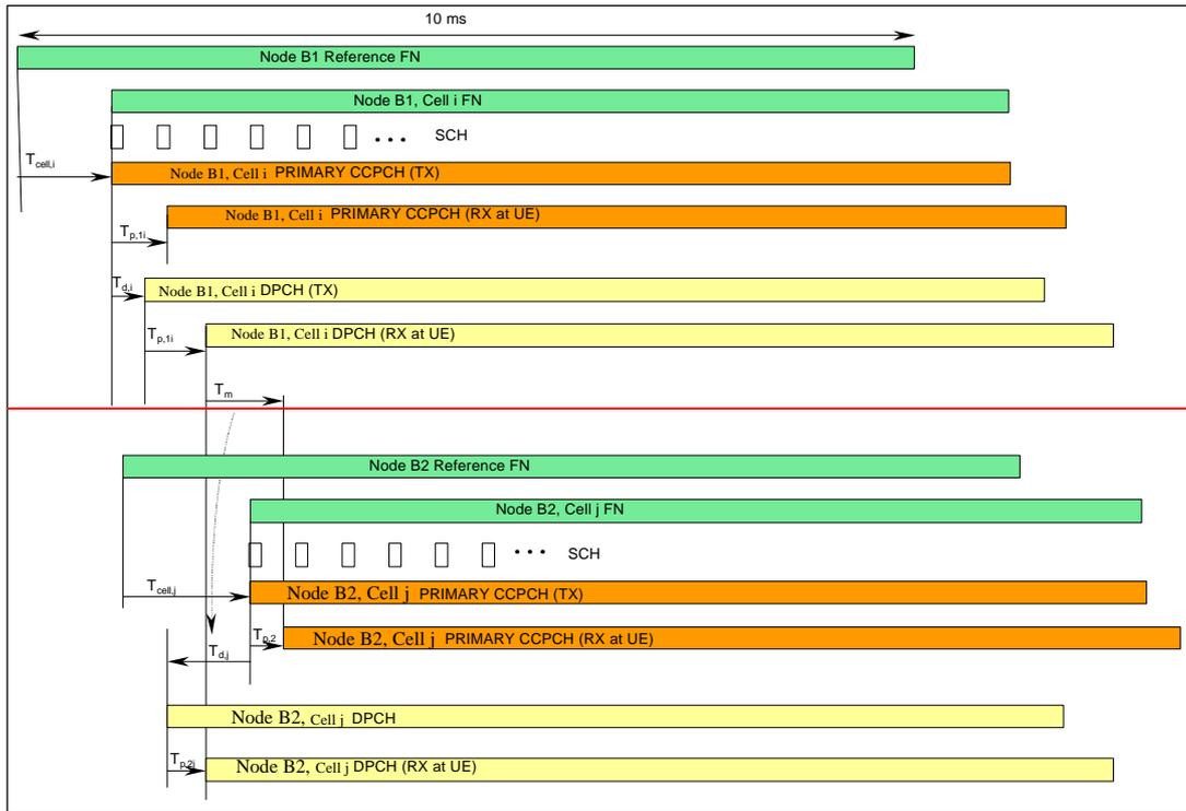
**Figure 10. Physical channel timing parameters**
