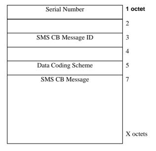
Figure 6.12: SMS CB message format (RLC SDU)
