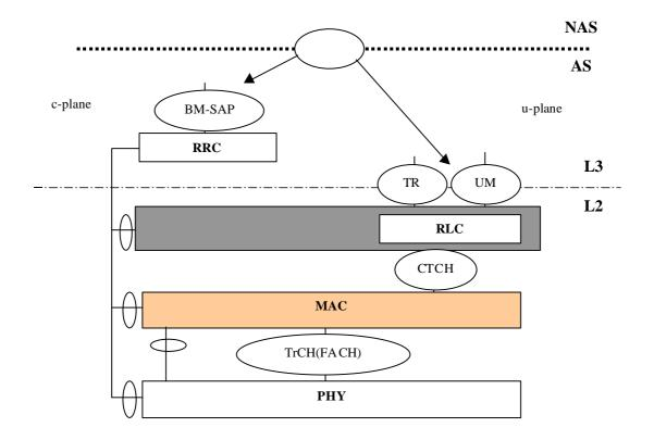
Figure 6.n: Detailed protocol architecture of option 3
