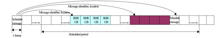
Figure 6.13 SMS CB transmission scenario
