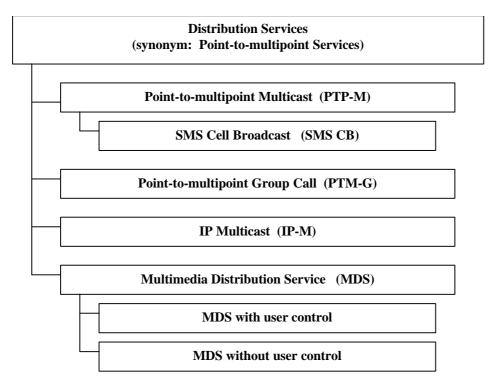
Figure 1: Structure of point-to-multipoint services
