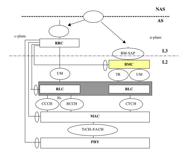
Figure 6.n: Detailed protocol architecture of option 1
