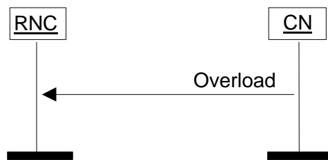
Figure 13138. Overload at the CN.
