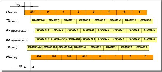
Figure 9. Radio interface downlink synchronisation (2)
