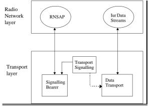
Figure 17. Separation of RNSAP and transport over lur
