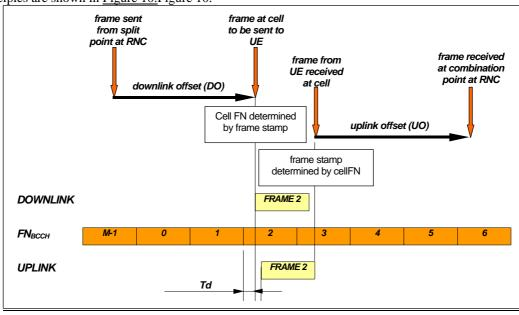
Figure 10. Frame stamping and uplink/downlink offsets handling
