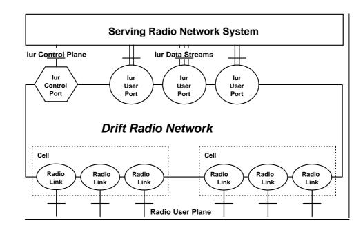
Figure 16. Drift RNS Logical Model
