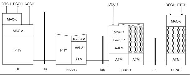
Figure 23. FACH: Separate Controlling and Serving RNC
