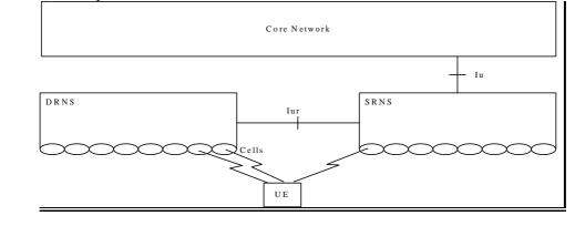
Figure 5. Serving and Drift RNS
