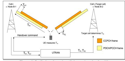
Figure 8. Radio interface downlink synchronisation (1)
