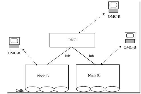
Figure 13.RNS architecture with O&M interfaces
