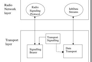
Figure 19. Separation of Radio Network protocols and transport over lub
