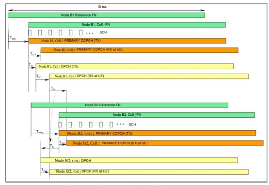
Figure 7. Physical channel timing parameters
