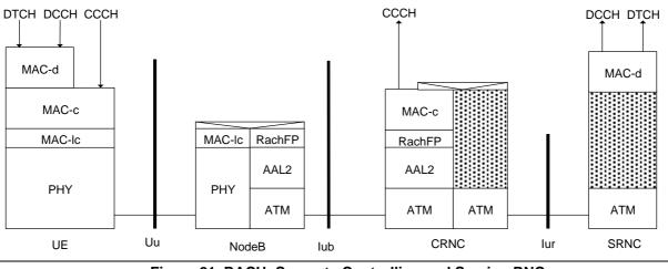
Figure 21. RACH: Separate Controlling and Serving RNC
