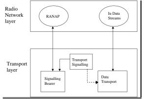
Figure 15. Separation of RANAP and transport over lu
