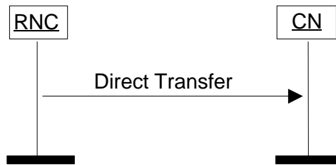
Figure 17 16 Figure 19 Figure 16 . Direct Transfer, RNC originated.
