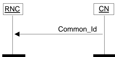
Figure 111310 . Common Id procedure.
