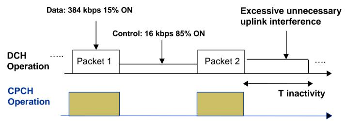
•When Compared to CPCH, DCH Control Channel
