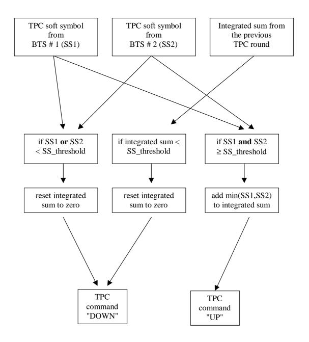
Figure 2. Flowchart of the INT algorithm operation, in a case where the INT is used in parallel with SS algorithm. The INT algorithm cannot be employed unless parallel to another algorithm block.
