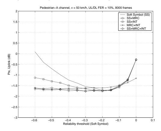
Figure 14. Comparison of TPC algorithms listed in Table 1. Mobile speed is 50 km/h, UL/DL FER is 10%.
