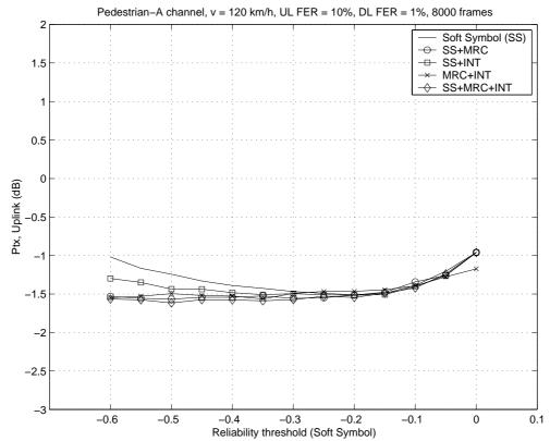
Figure 18. Comparison of TPC algorithms listed in Table 1. Mobile speed is  $120 \, \text{km/h}$ , UL FER is 10% and DL FER is 1%.
