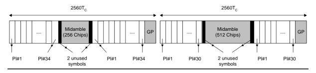
Figure 16: Example of PI Transmission in the PICH bursts of different types for Lpi=4
