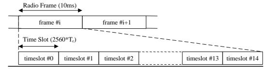
Figure 1: Physical channel signal format
