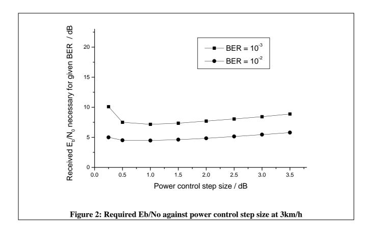
In this more slowly-changing environment, there is also some degradation if the step size is made too large, as the power control steps themselves start to be the cause of SIR errors in the uplink. The effect of errors in the interpretation of the power control bits by the mobile terminal is also more severe if the step size is too large.
