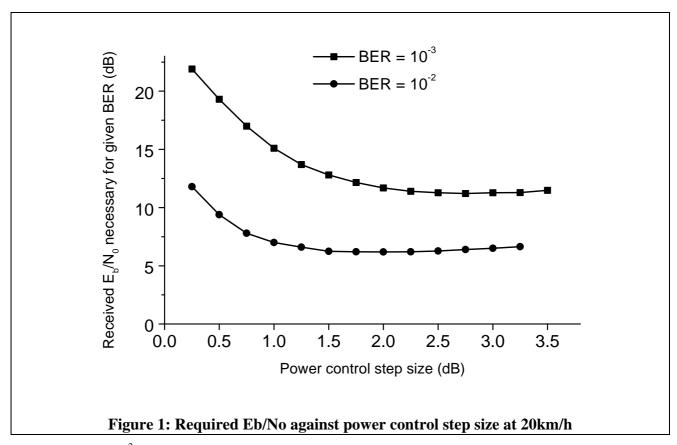
For a BER of  $10^{-3}$ , a 3.5dB gain in required  $E_b/N_0$  can be obtained by using a 2dB step size instead of 1dB.
