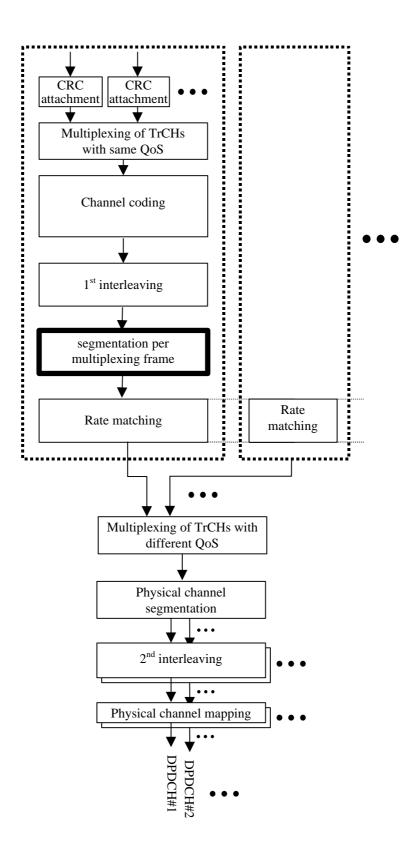
Figure 2 Transport channel multiplexing structure for FDD uplink.
