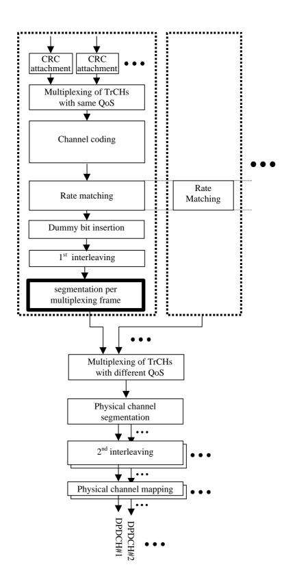
Figure 3 Transport channel multiplexing structure for TDD downlink and TDD uplink.
