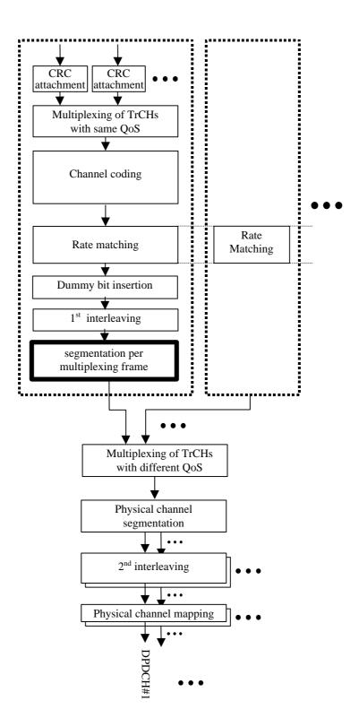
Figure 1 Transport channel multiplexing structure in FDD downlink.
