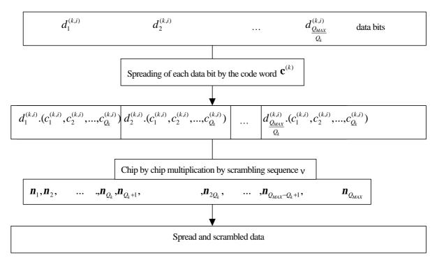
Figure 3: Spreading and subsequent scrambling of data bits.
