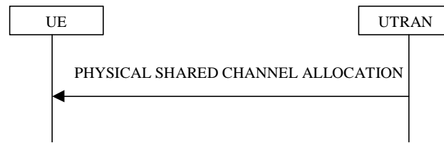
Figure 8.2.7-1: Physical Shared Channel Allocation
