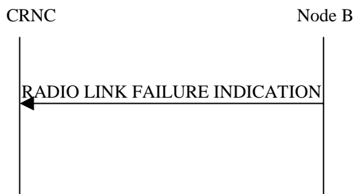
Figure 43: Radio Link Failure procedure, Successful Operation
