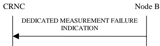
Figure 42: Dedicated Measurement Failure procedure, Successful Operation
