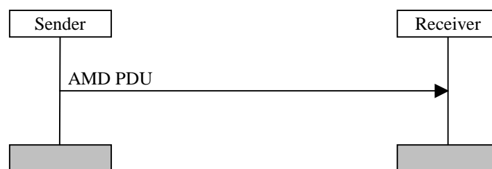
Figure 11.3: Acknowledged mode data transfer procedure
