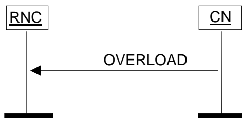
Figure 29: Overload at the CN.
