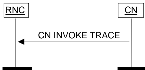
Figure 1: CN Invoke Trace procedure
