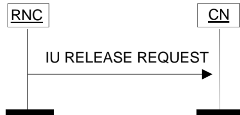
Figure 1: Iu Release Request procedure. Successful Operation
