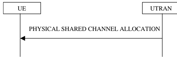
Figure 29: Physical Shared Channel Allocation
