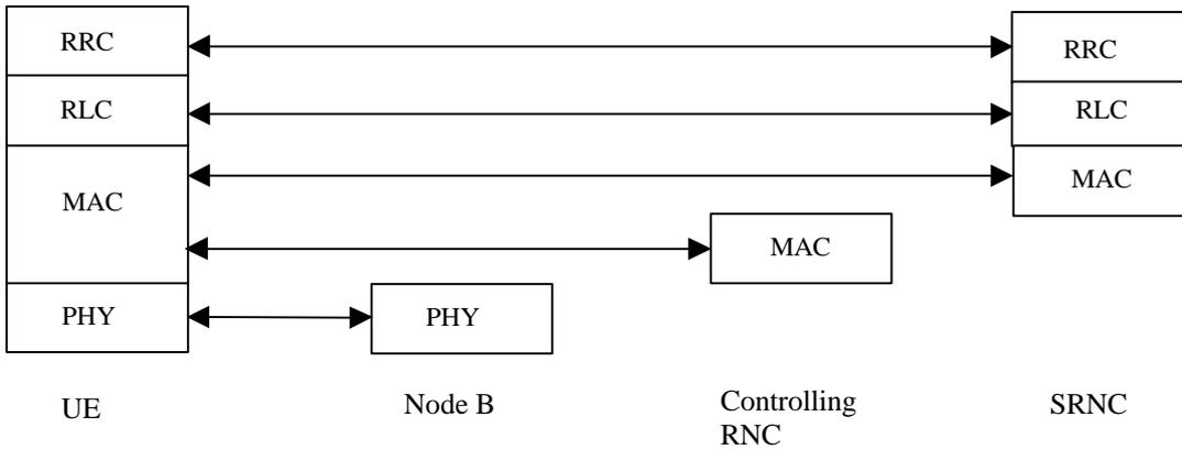
**Figure 14: Protocol Termination for RACH/FACH, control plane**
