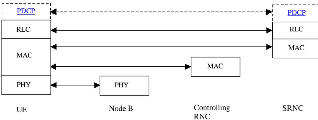
**Figure 15: Protocol Termination for RACH/FACH, user plane**
