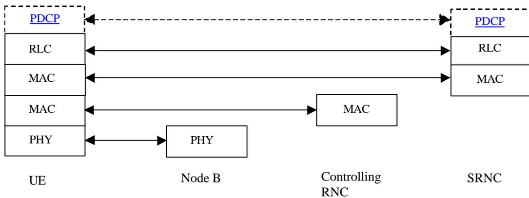
Figure 18: Protocol termination points for DSCH, user plane.
