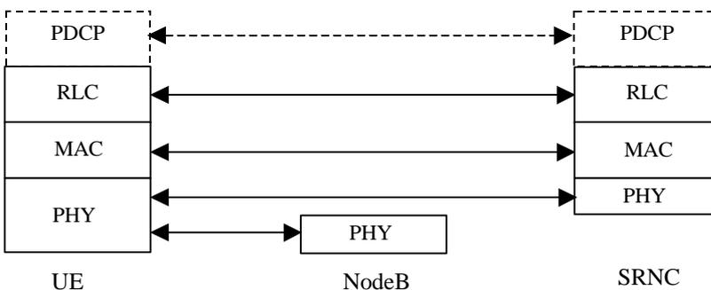
**Figure 13: Protocol Termination for DCH, user plane**
