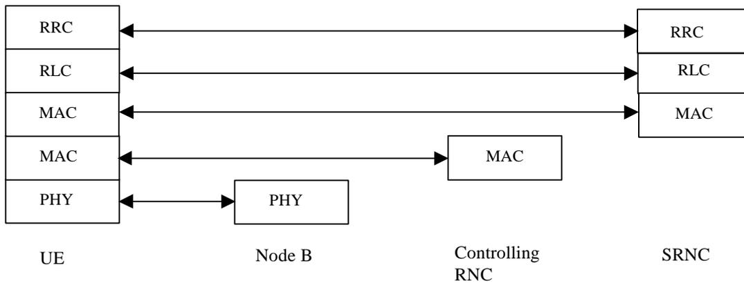
Figure 17: Protocol termination points for DSCH, control plane.
