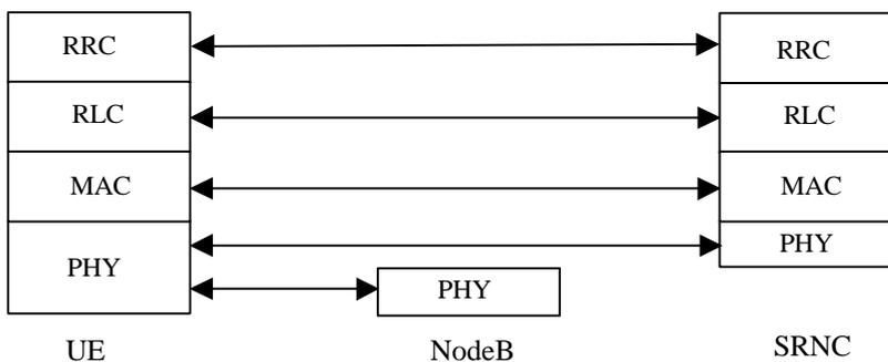
**Figure 12: Protocol Termination for DCH, control plane**
