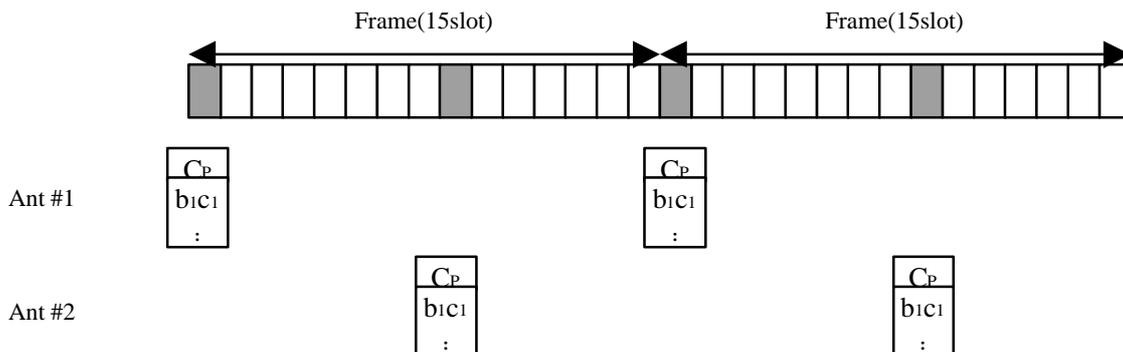
Figure 5. Antenna Switching Pattern (Case 2)
