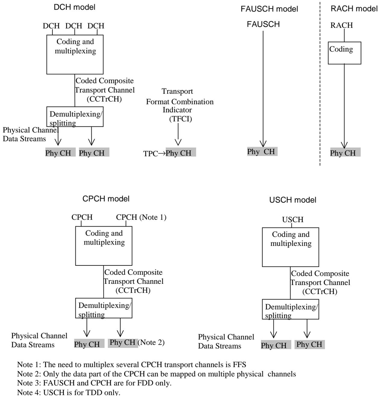
**Figure 1: Model of the UE's physical layer – uplink**
