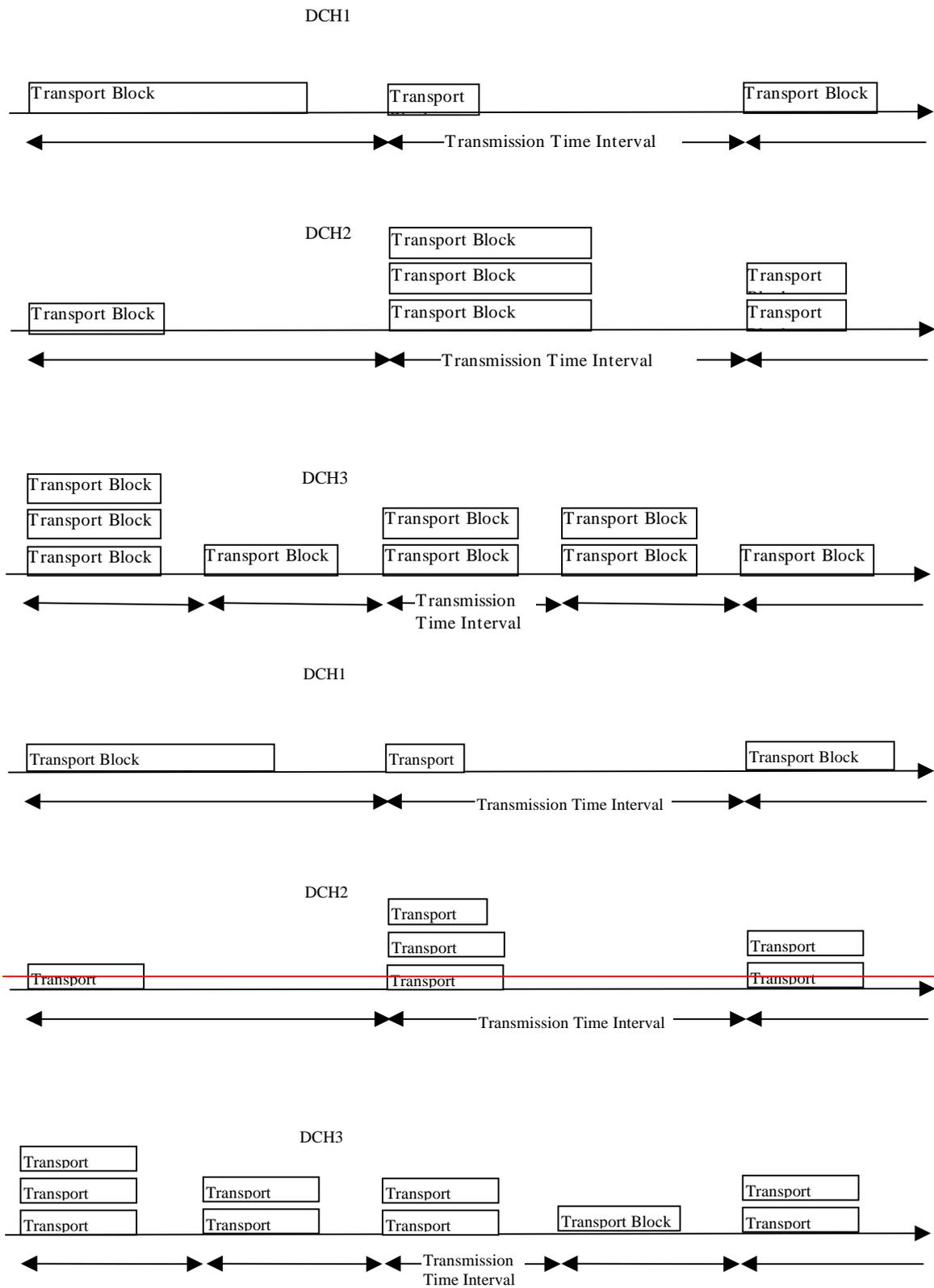
Figure 1. Exchange of data between MAC and L1
