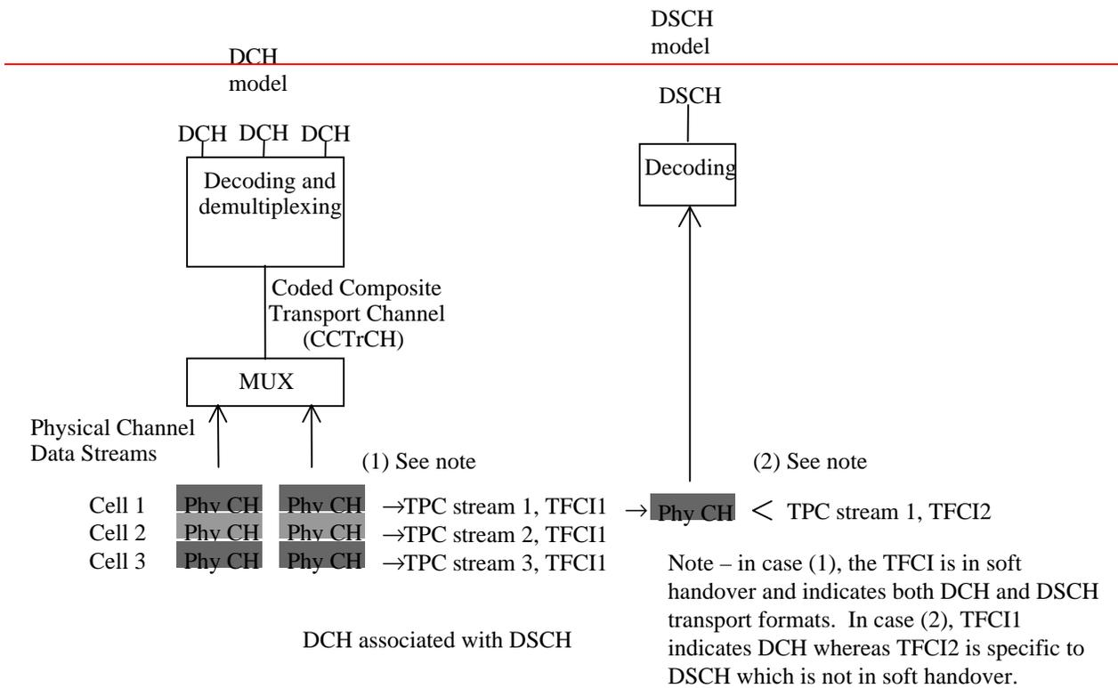
**Figure 2: Model of the UE's physical layer – downlink FDD mode**
