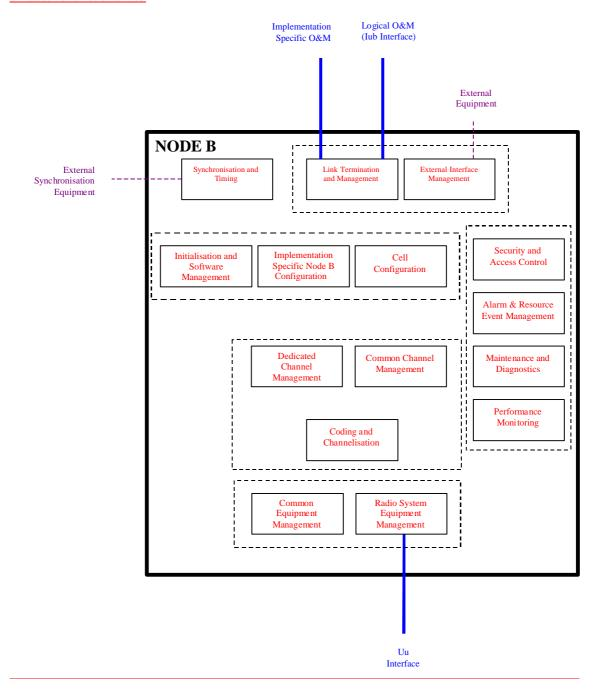
[Note] The Logical O&M (Iub interface) and Implementation Specific O&M interface are represented above as logically independent interfaces. It should be possible to route both the Iub interface and Implementation Specific O&M interface either independently or via the same physical bearer.
