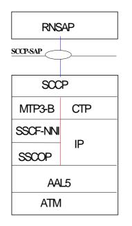
Fig.3 Signalling bearer for RNSAPAlternative 3
