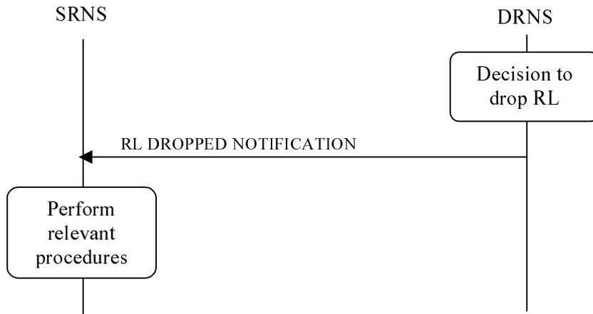
Figure 9-11. RL Dropped Notification procedure
