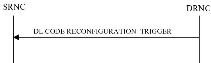
Figure 9-7. An example RNSAP message flow at I<sub>ur</sub> interface for DL Code Reconfiguration Trigger
