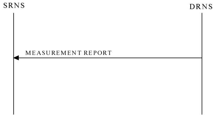
Figure 9-12. Radio Measurements Reporting
