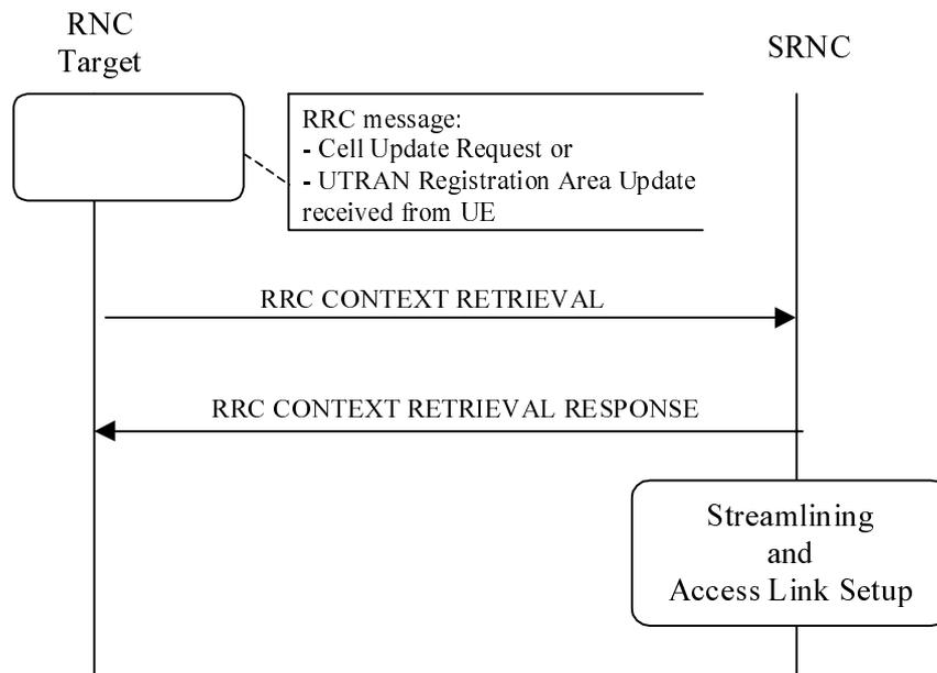
Figure 9-10. An example RNSAP message flow at I<sub>ur</sub> interface for RNC Relocation (Forward method)
