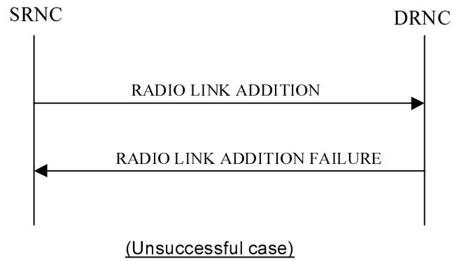
Figure 9-2. An example RNSAP protocol message flow at I<sub>UR</sub> interface for inter RNS RL addition.
