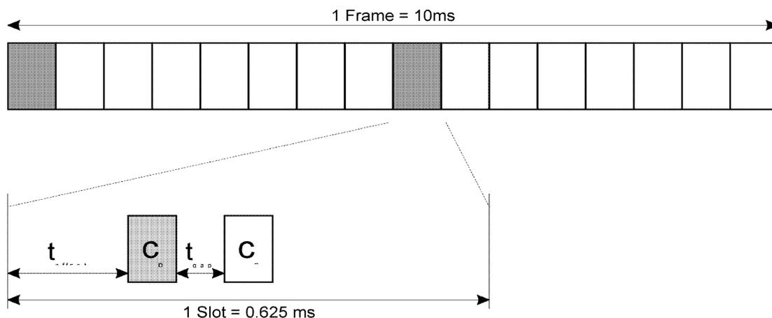
**Figure 1: Structure of synchronisation channel (SCH)**
