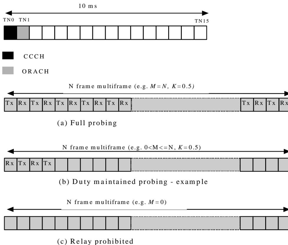
**Figure 2: Probing state machines and mechanism**
