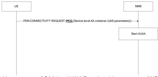
C1-216134 enables transport of CAA-level UAV ID and enables transport of USS address, if CAA-level UAV ID and USS address are small enough to fit into PCO IE, during attach procedure.
