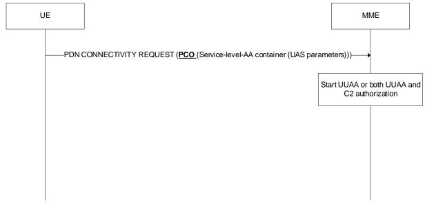
Solution enables transport of CAA-level UAV during attach procedure.
