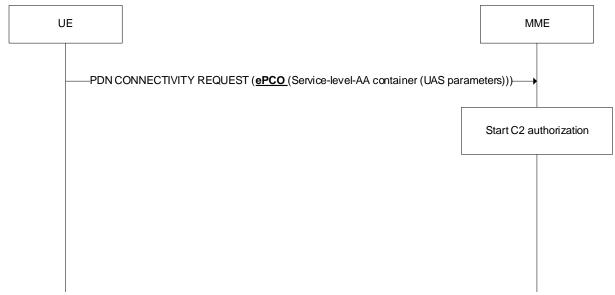
Solution requires changes of MME to consider ePCO IE of PDN CONNECTIVITY REQUEST, of IP based PDN connection in WB-S1 mode, as valid IE and handle it accordingly
