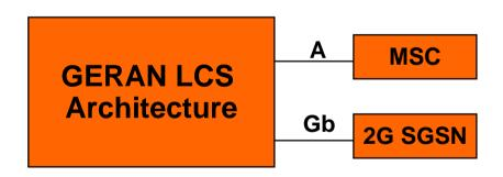
1. A/Gb mode: LCS support on packet-data channels and over the A/Gb interface.
