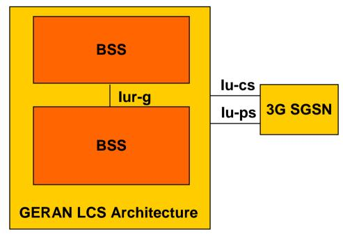
2. Iu mode: LCS support over the Iu-ps, Iu-cs, Iur-g interfaces.
