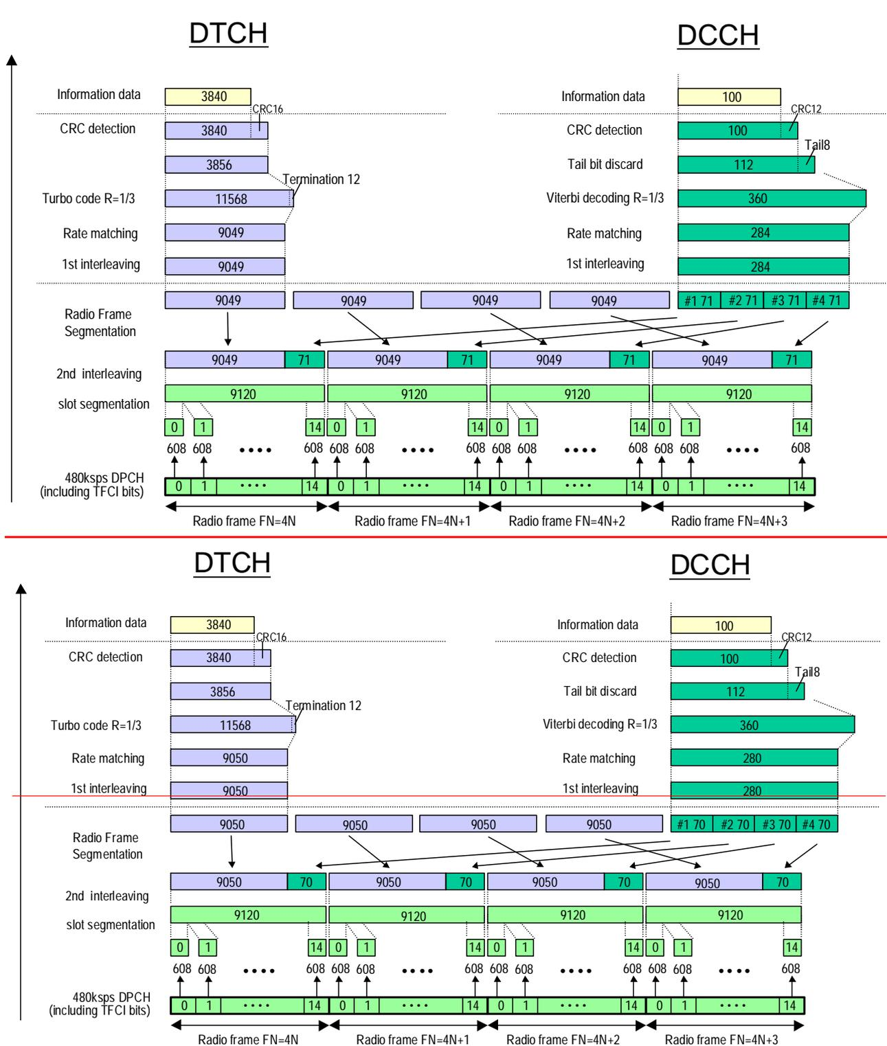
Figure C.3.45 (Informative): Channel coding of DL reference measurement channel (384 kbps)
