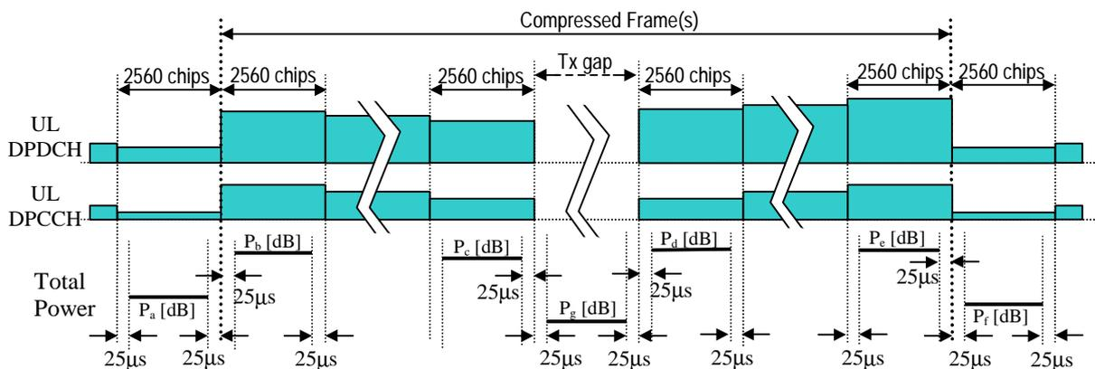
**Figure 5.7.4: Uplink transmit power in uplink compressed mode**
