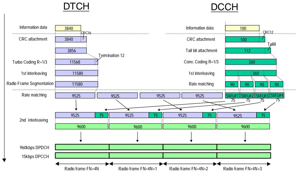
Figure C.2.45 (Informative): Channel coding of UL reference measurement channel (384 kbps)
