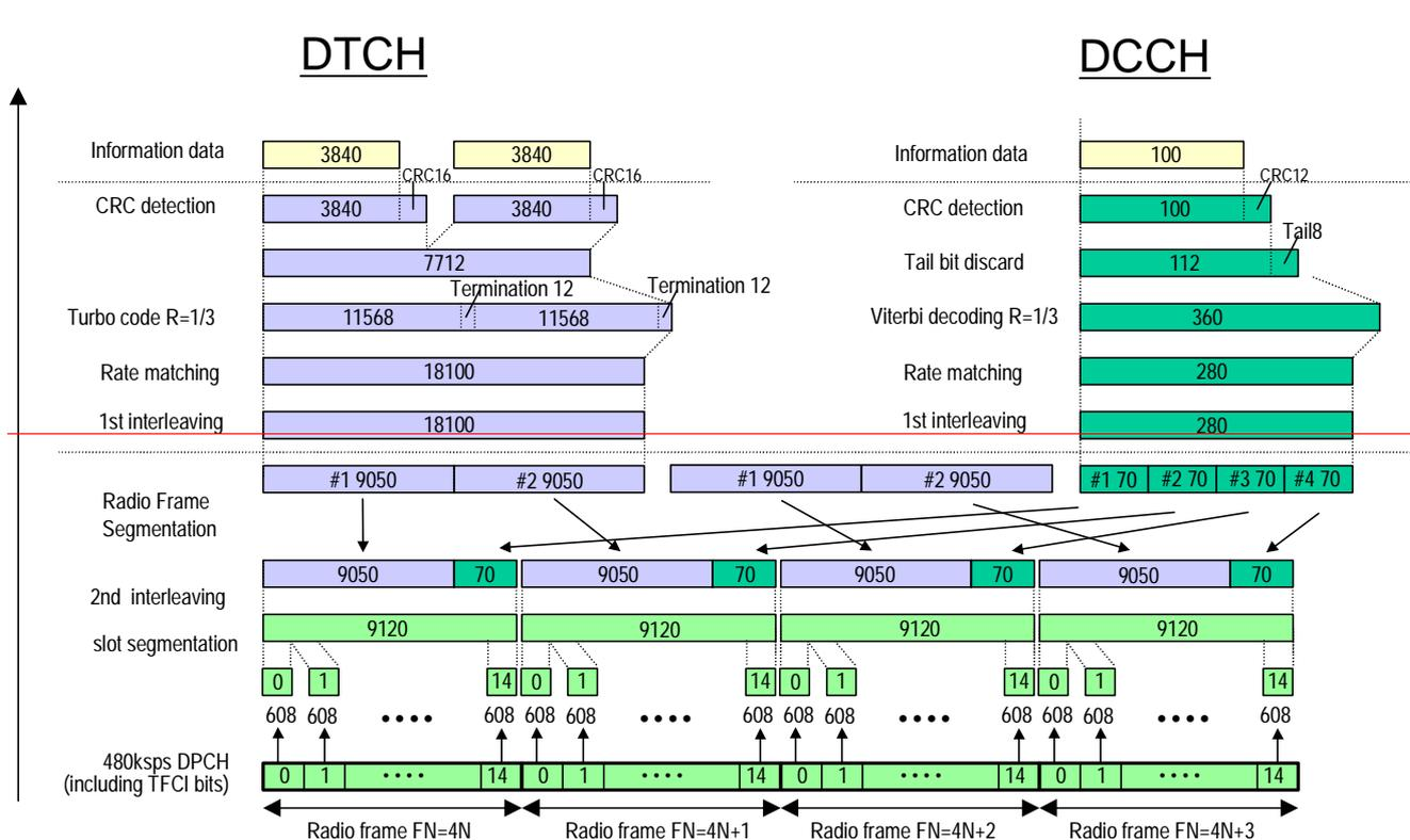
**Figure C.3.4 (Informative): Channel coding of DL reference measurement channel (384 kbps, 20ms TTI)**
