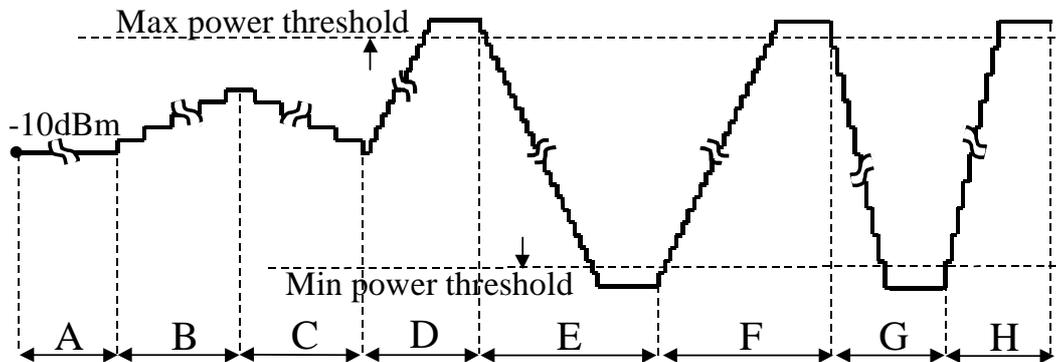
Figure 5.4.2.4 Inner Loop Power Control Test Steps
