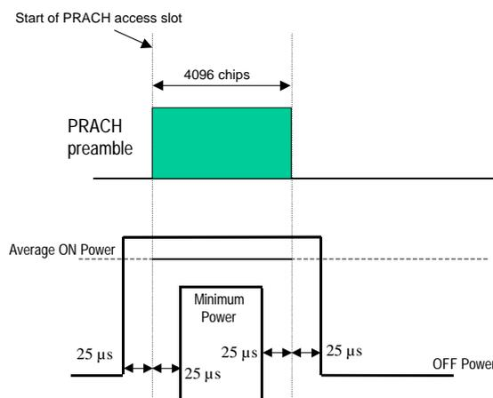
**Figure 5.5.1: Transmit ON/OFF template for PRACH preambles**
