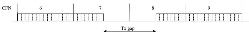
**Figure 5.7.3: Pattern B for compressed mode test**
