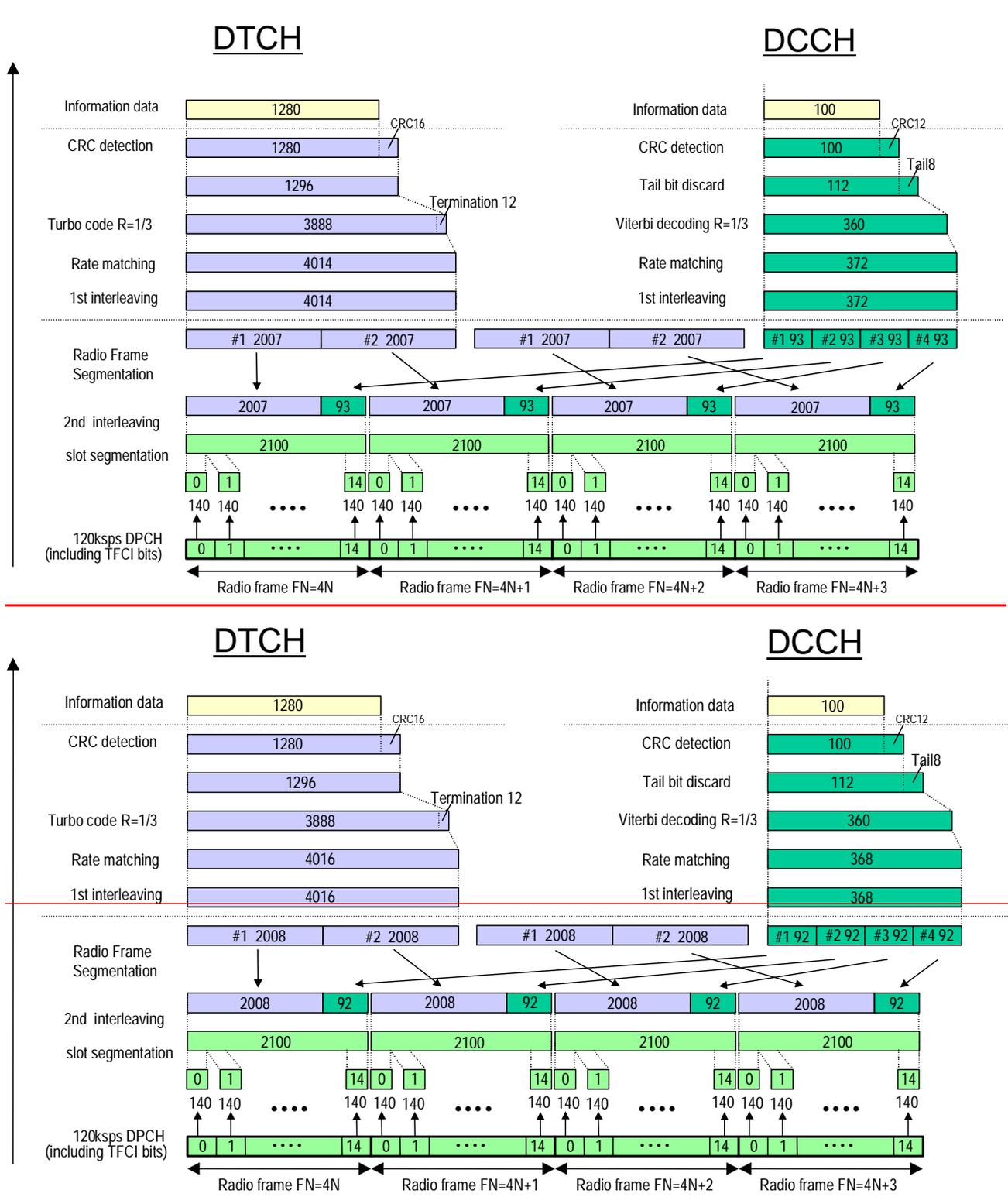
Figure C.3.2 (Informative): Channel coding of DL reference measurement channel (64 kbps)
