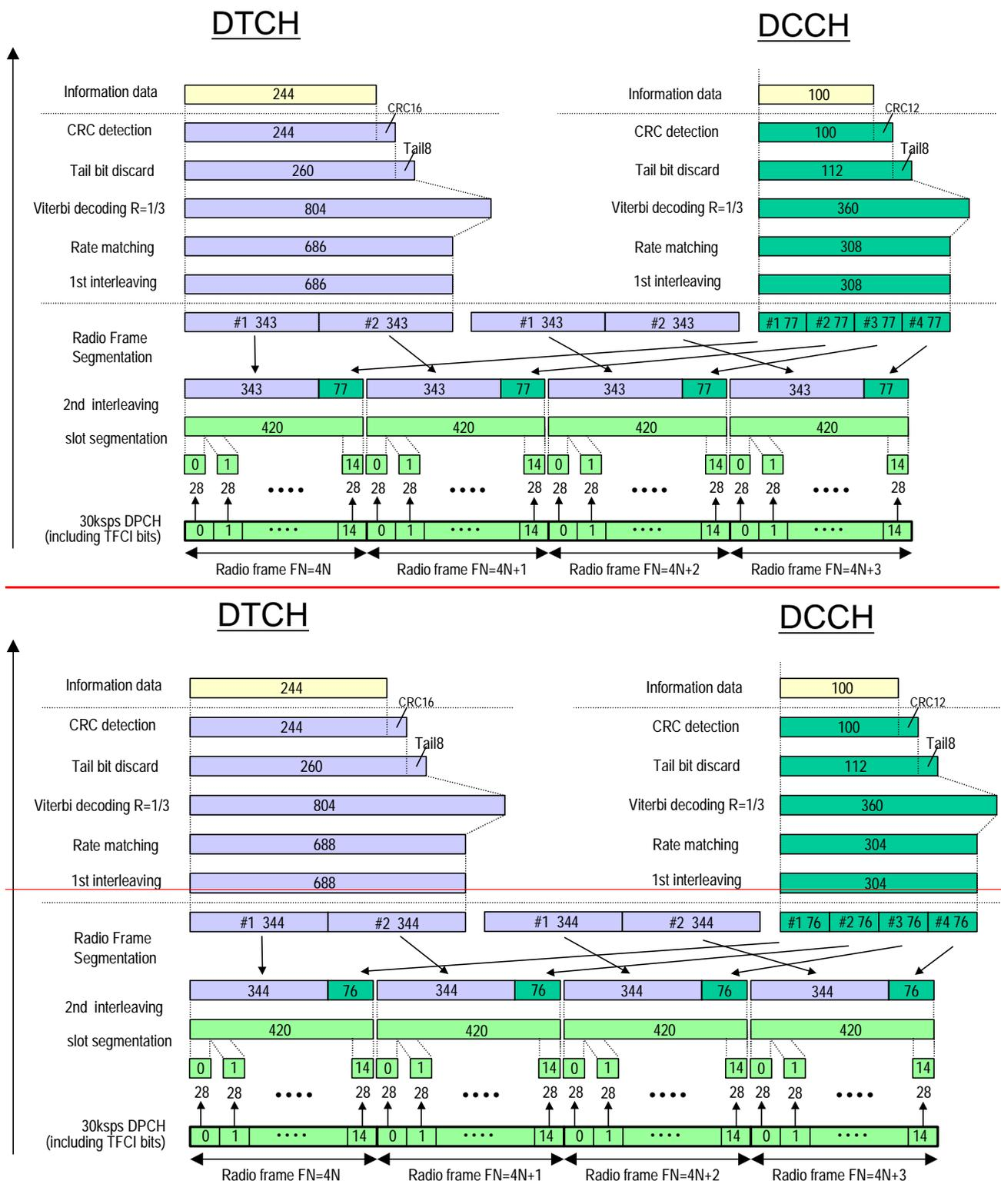
Figure C.3.1 (Informative): Channel coding of DL reference measurement channel (12.2 kbps)
