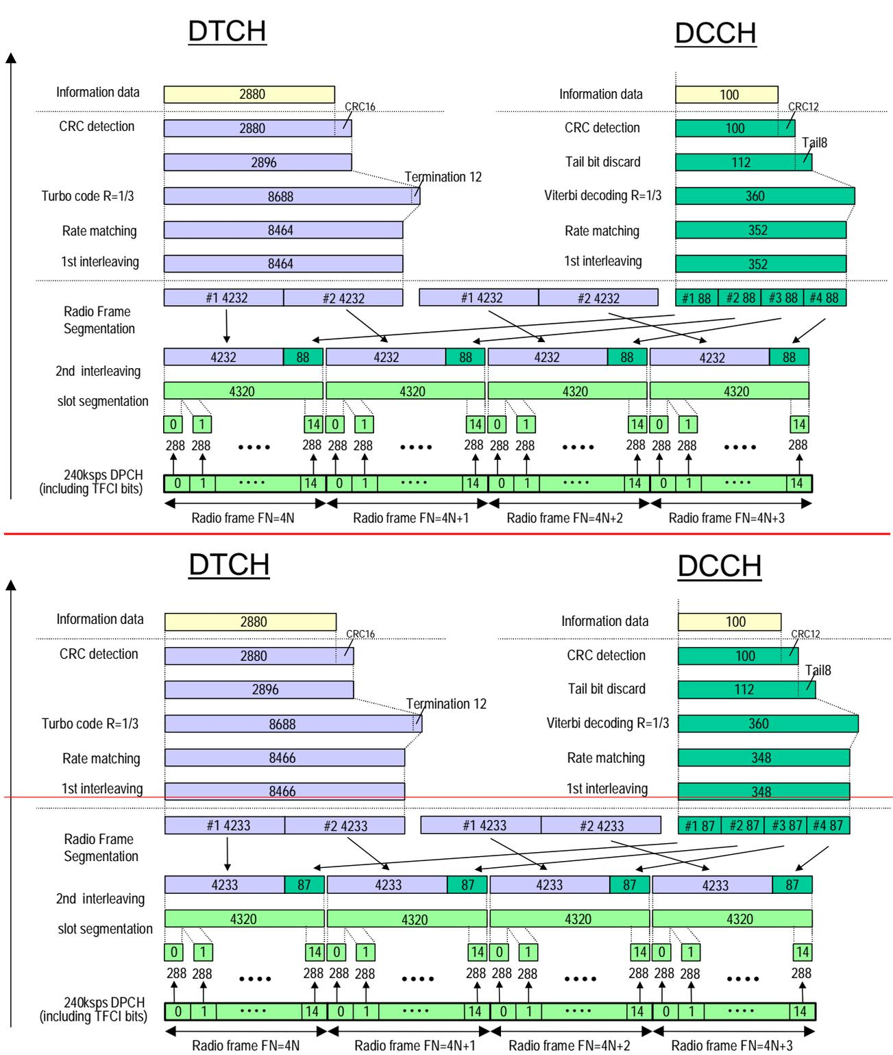
Figure C.3.3 (Informative): Channel coding of DL reference measurement channel (144 kbps)
