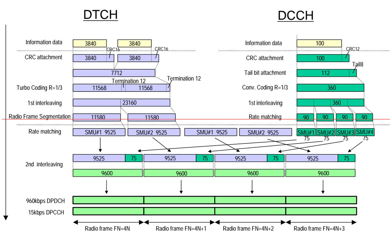
**Figure C.2.4 (Informative): Channel coding of UL reference measurement channel (384 kbps, 20ms TTI)**
