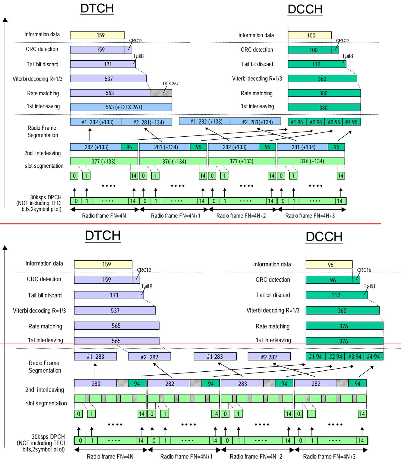
Figure C.4.2 (Informative): Channel coding of DL reference measurement channel for BTFD (Rate 2)
