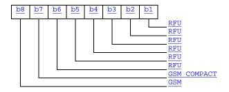
The RFU bits are coded with '0' in the bit positions.
