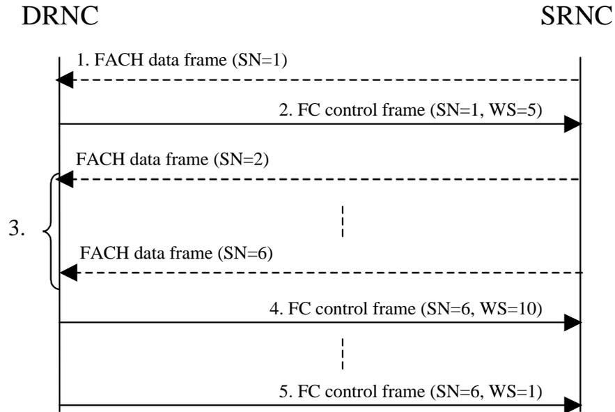
Figure 2-1. Example of u-plane signalling for FACH data streams o/Iur.
