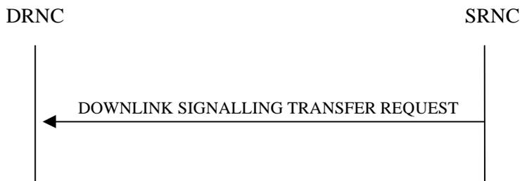
Figure 9-9: An example RNSAP message flow at I<sub>ur</sub> interface for Downlink Signalling Transfer
