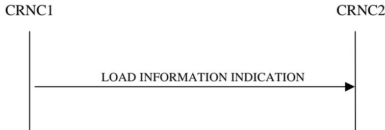
Figure 9-x: An example RNSAP message flow at I<sub>ur</sub> interface for Load Information.
