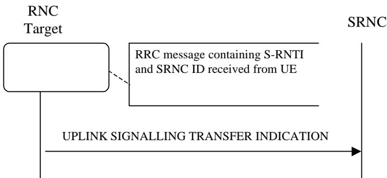
Figure 9-8: An example RNSAP message flow at I<sub>ur</sub> interface for Uplink Signalling Transfer
