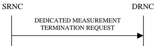
Figure 9-x: Measurement Termination Procedure initiated by SRNC
