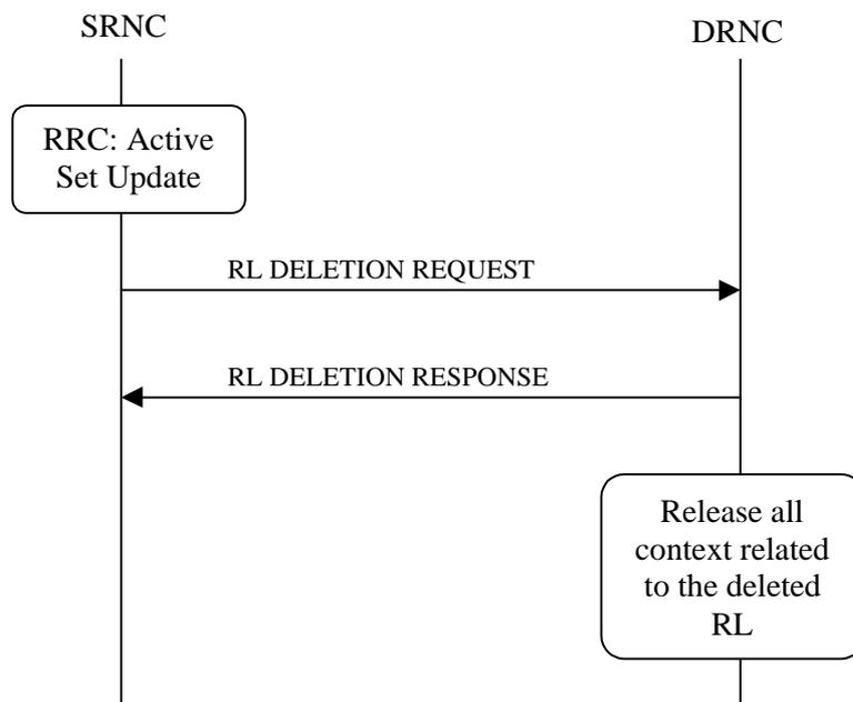
Figure 9-3. An example RNSAP protocol message flow at I<sub>ur</sub> interface for interRNS RL deletion.
