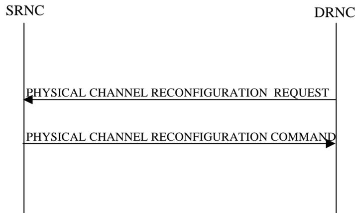
Figure 9-6. Physical Channel Reconfiguration procedure
