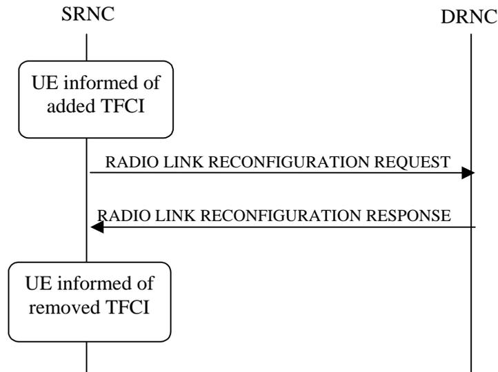
Figure 9-5. RL Reconfiguration procedure (unsynchronised)
