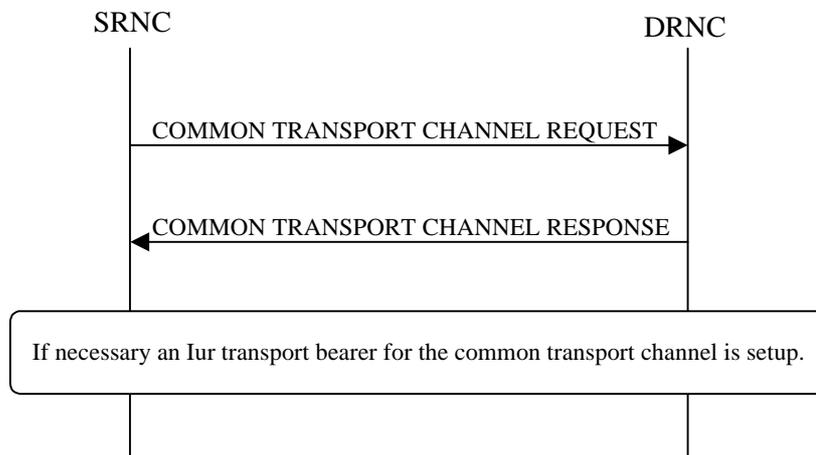
Figure 9-x. An example RNSAP message flow at I<sub>ur</sub> interface for Common Transport Channel Initialization.
