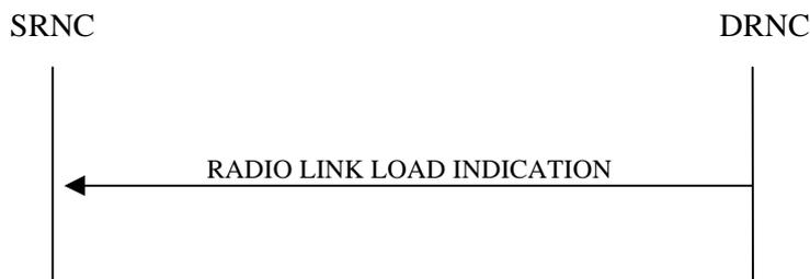
Figure 9-x: An example RNSAP message flow at I<sub>ur</sub> interface for Radio Link Load Indication.
