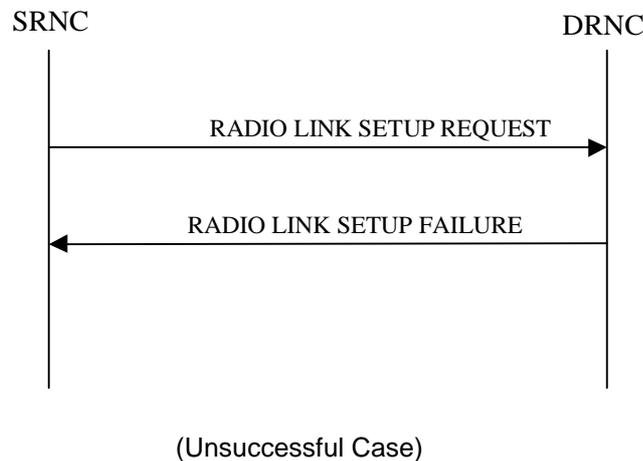
Figure 9-1. An example RNSAP message flow at I<sub>ur</sub> interface for RL setup.
