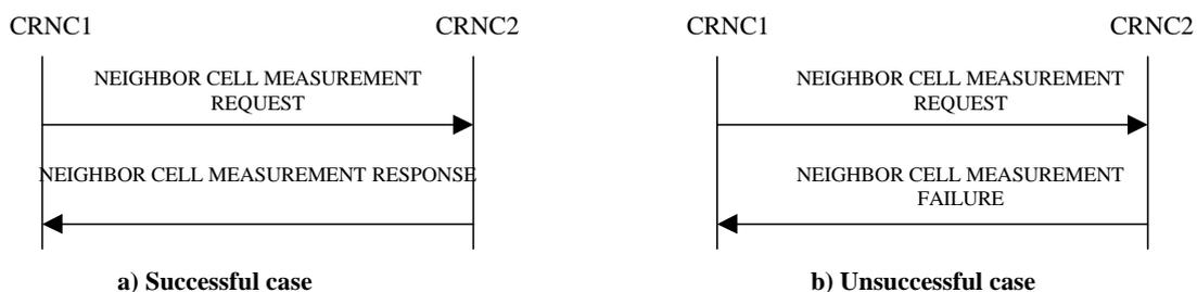
Figure 9-x: An example RNSAP message flow at I<sub>ur</sub> interface for Neighbour Cell Measurement.
