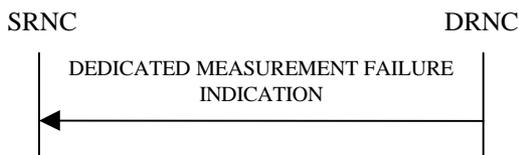
Figure 9-x: Measurement Termination Procedure initiated by DRNC
