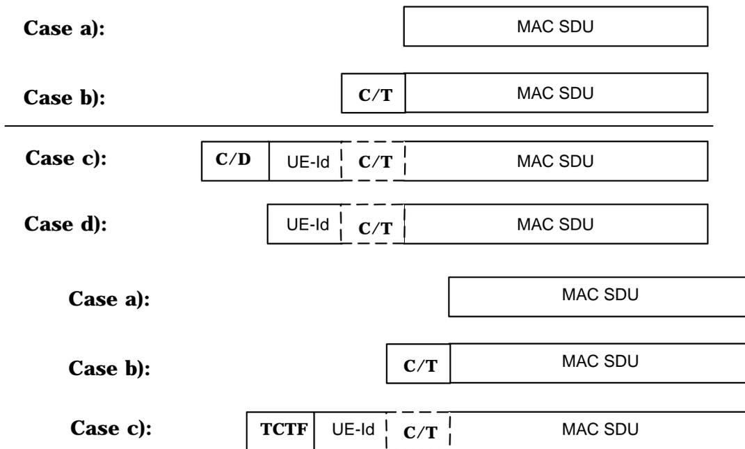
**Figure 9.2.2.1: MAC Data PDU formats for DTCH and DCCH**
