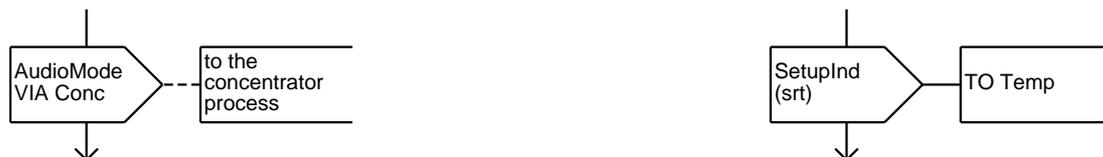
Figure 51: Examples of the use of TO and VIA.
