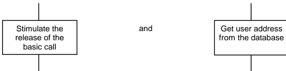
This notation is very easy to understand but it is not possible simulate or validate the action in the symbol. According to the strict definition of SDL, the text, "Stimulate the release of the basic call", is interpreted as a name at the start of an incomplete, and therefore incorrect, assignment statement. To make such expressions formal and executable, *convert informal text descriptions of actions into procedure calls and replace the task symbols with a procedure symbols*, thus:
