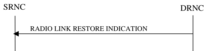
Figure 6: RL Restoration procedure, Successful Operation
