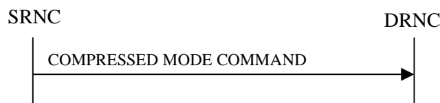
Figure 26: Compressed Mode Command procedure, Successful Operation
