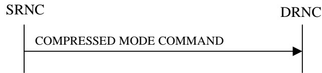
Figure 26: Compressed Mode Command procedure, Successful Operation
