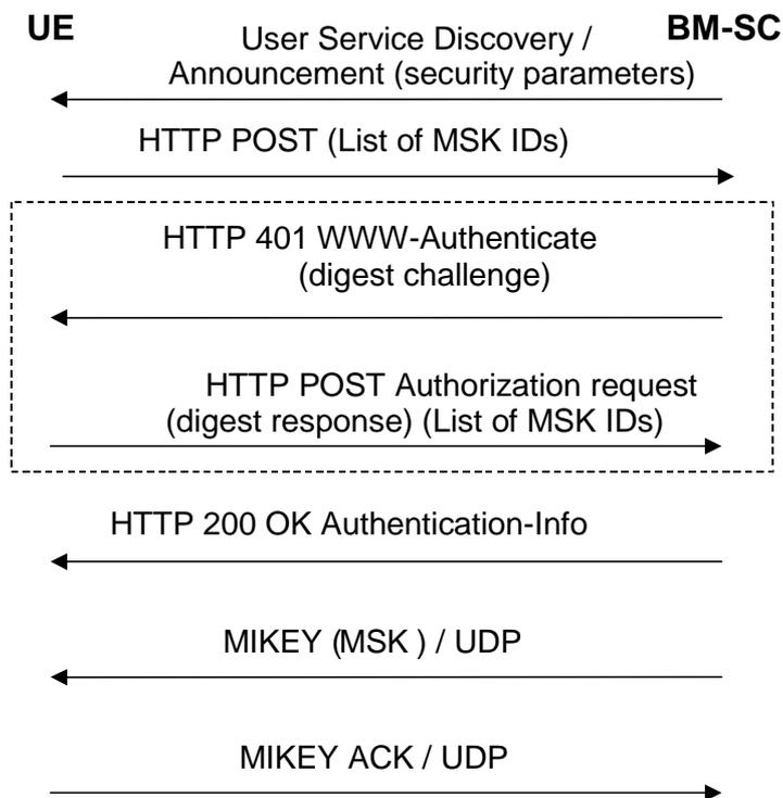
Figure 6.2a: MSK retrieval procedure
