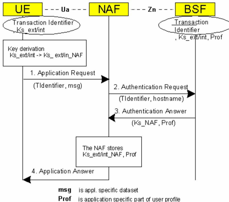
Figure 5.3: The bootstrapping usage procedure with UICC-based enhancements
