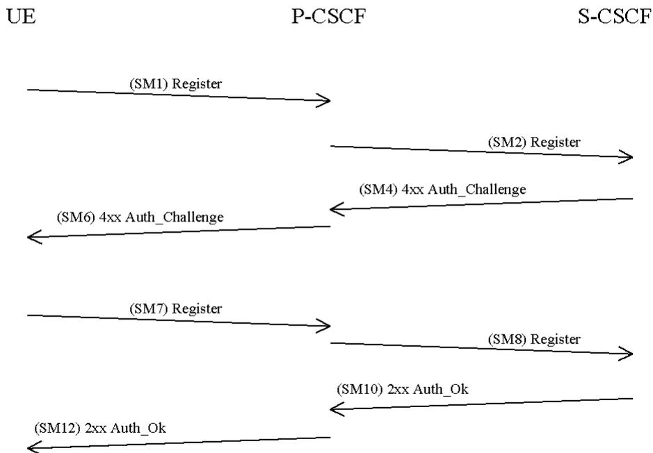
The UE sends a Register message towards the S-CSCF to register the location of the UE and to set-up the security mode, cf. clause 6.1. In order to start the security mode set-up procedure, the UE shall include a *Security-setup*-line in this message. The *Security-setup*-line in SM1 contains the SPIs and the numbers and of the protected ports assigned selected by the UE for the SAs for TCP and UDP. It also contains a list of identifiers for the integrity algorithms which the UE supports.
