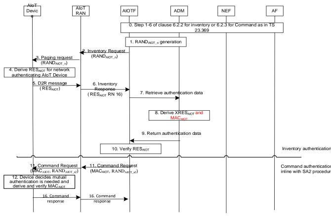
8. knowing it's command procedure and mutual authentication procedure is needed ADM shall derive  $MAC_{AIOT}$  using  $K_{AIoT}$  and  $RAND_{AIOT\_n2}$  for device authenticating network. This step could happen after step 7 and before step 9.
