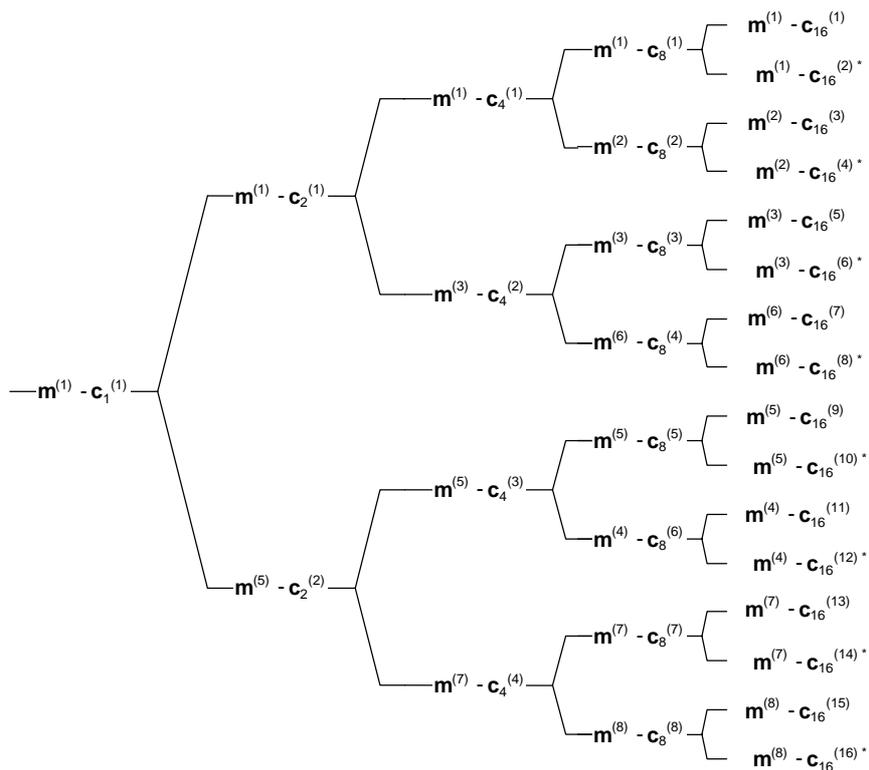
Figure A-2A.2: Association of Midambles to Spreading Codes for Burst Type 1/3 and  $K_{Cell}=8$
