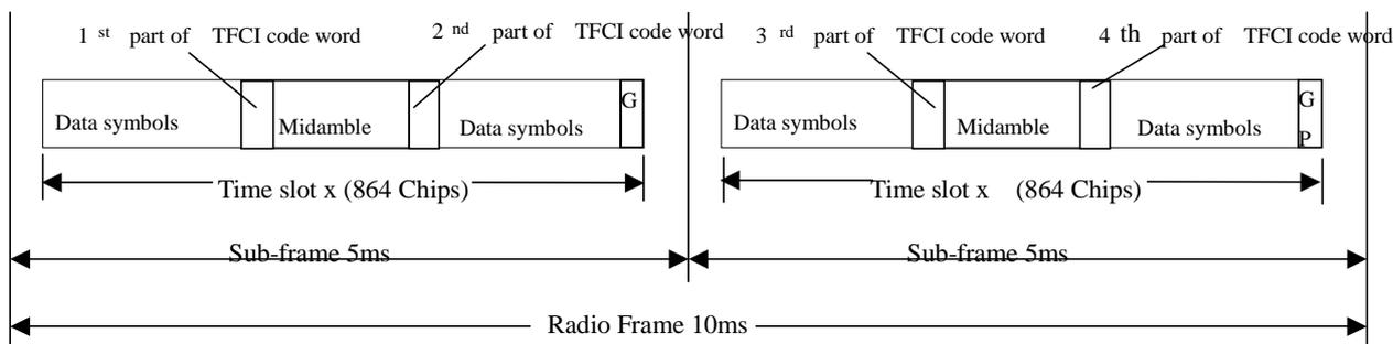
**Figure 23.18E: Position of the TFCI code word in the traffic burst in case of no TPC and SS in 1.28 Mcps TDD**
