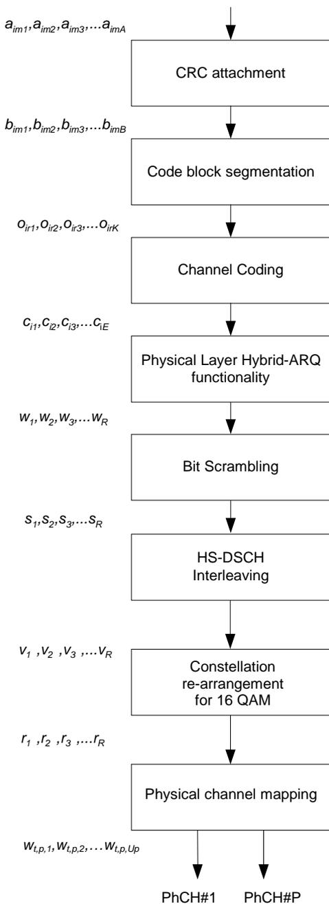
**Figure 4.6.15. Coding chain for HS-DSCH**
