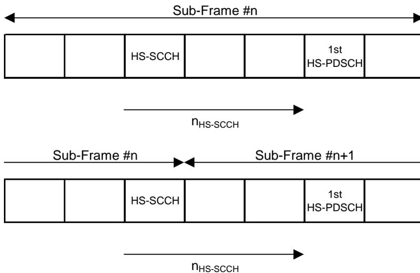
Figure 2437: Timing for HS-SCCH and HS-DSCH for different radio frame configurations for a given UE
