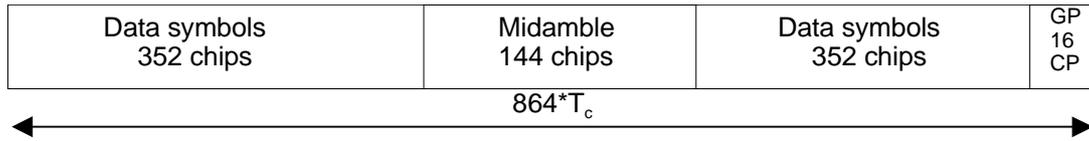
Figure 18D22: Burst structure of the traffic burst format (GP denotes the guard period and CP the chip periods)
