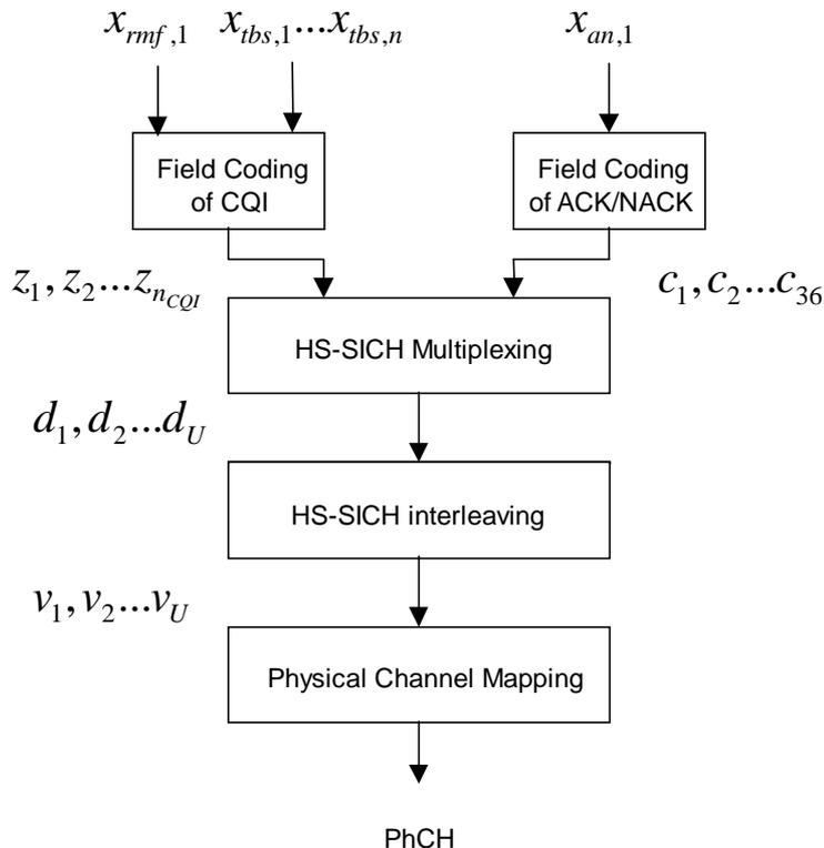
Figure [2019](#) Coding and multiplexing for HS-SICH
