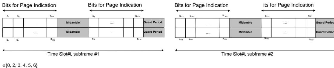
**Figure 2918K: Transmission and numbering of paging indicator carrying bits in the PICH bursts**
