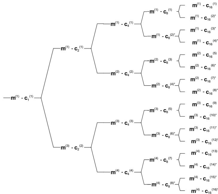
Figure AAB.2.7: Association of Midambles to Spreading Codes for K=4
