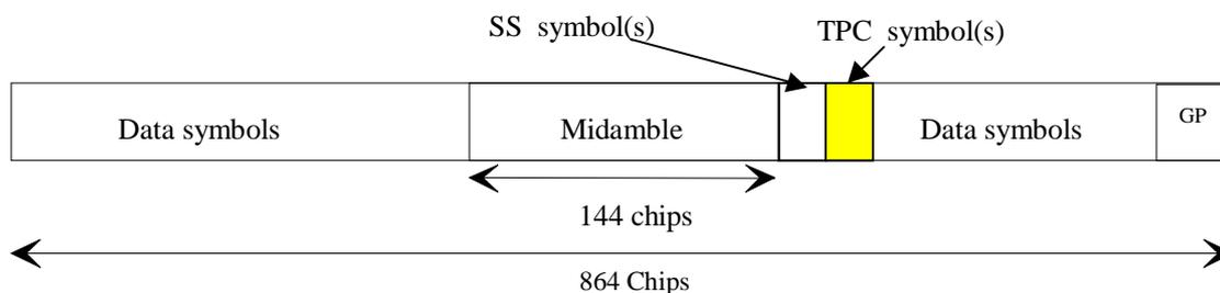
**Figure 18G25: Position of TPC information in the traffic burst in downlink and uplink**
