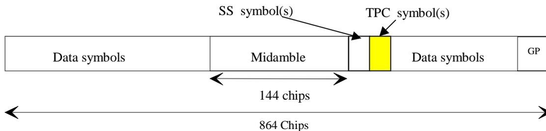
**Figure 25.18G: Position of TPC information in the traffic burst in downlink and uplink**
