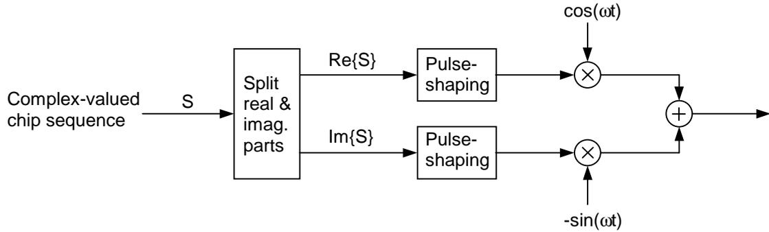
**Figure 3: Modulation of complex valued chip sequences**
