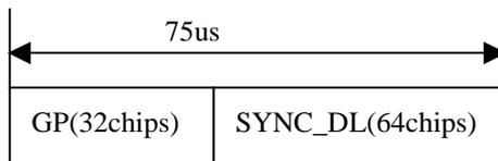
Figure 18J27: burst structure of the DwPCH ( DwPTS)
