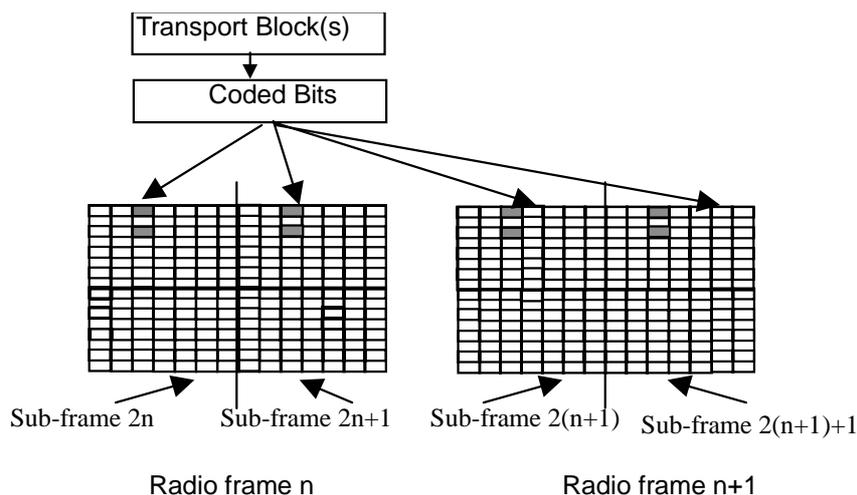
Figure 2336 : Mapping of Transport Blocks onto the physical bearer ( TTI= 20ms )
