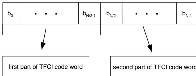
**Figure 89: Mapping of TFCI code word bits to timeslot**
