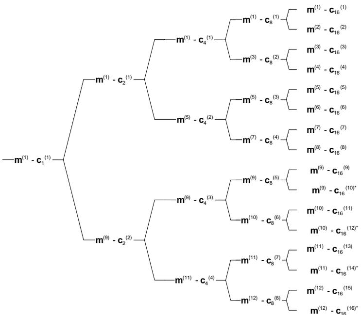
Figure AA.3B.2.3: Association of Midambles to Spreading Codes for K=12
