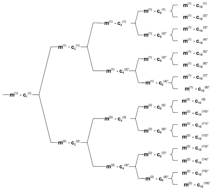
Figure AA.8B.2.8: Association of Midambles to Spreading Codes for K=2
