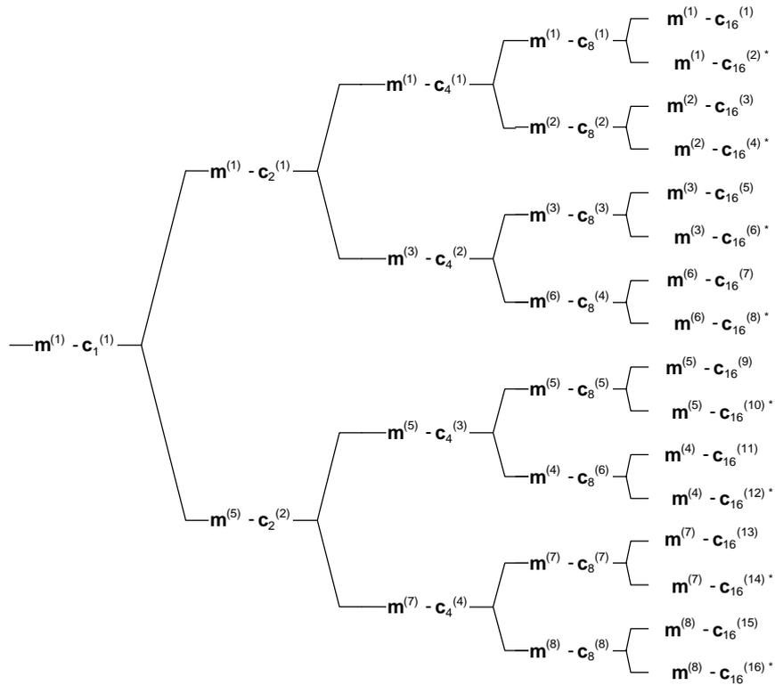
Figure A.3-2: Association of Midambles to Spreading Codes for Burst Type 1/3 and  $K_{Cell}=8$
