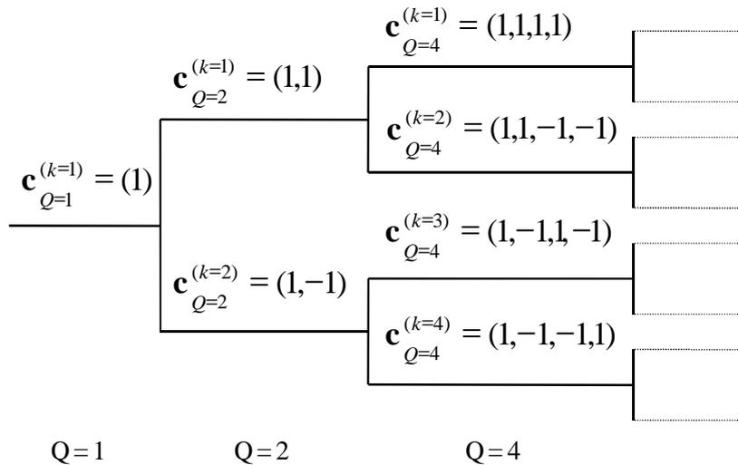
**Figure 1: Code-tree for generation of Orthogonal Variable Spreading Factor (OVVSF) codes for Channelisation Operation**
