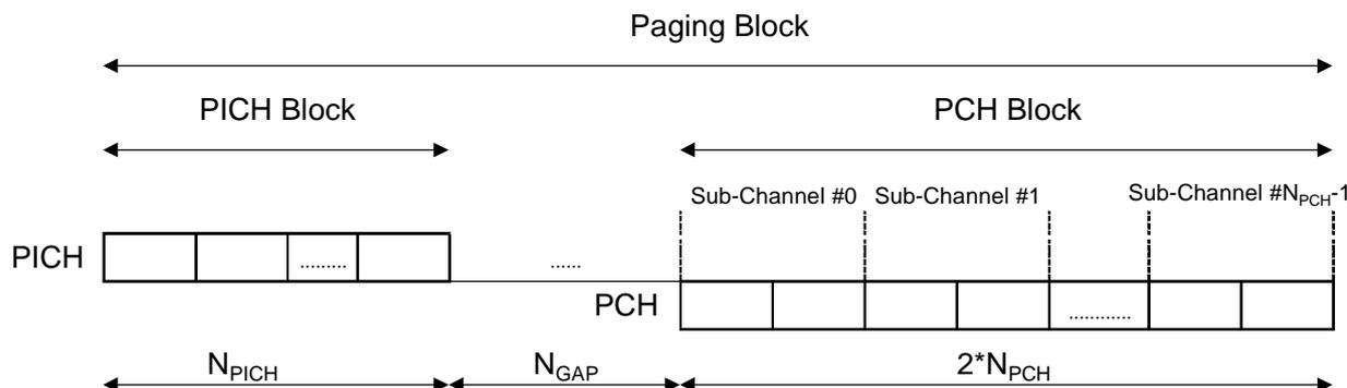
Figure 21.32: Paging Sub-Channels and Association of PICH and PCH blocks
