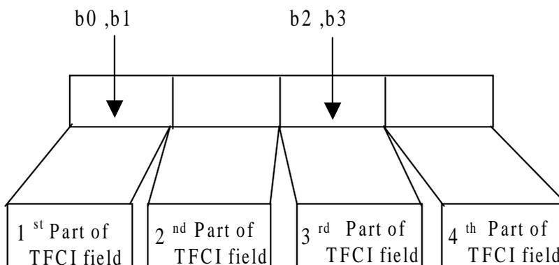
**Figure 1044: Mapping of TFCI code word bits to TFCI position in 1.28 Mcps TDD option, when  $N_{\text{TFCI code word}}=4$**
