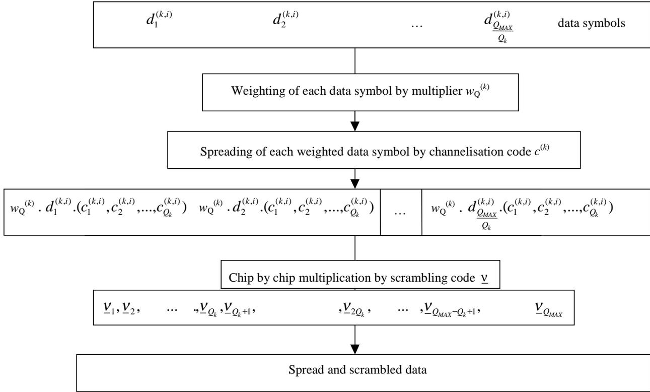
Figure 2: Spreading of data symbols
