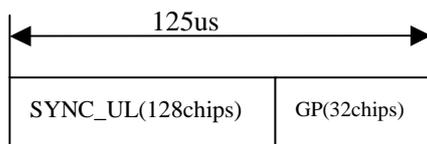
Figure 18J28: burst structure of the UpPCH ( UpPTS)
