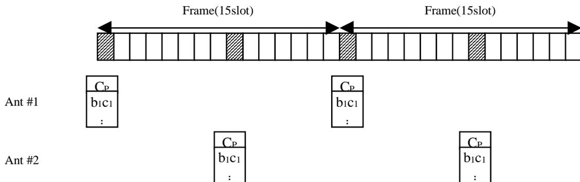
**Figure 3: Antenna Switching Pattern (Case 2)**
