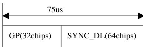
**Figure [2718I](#): burst structure of the DwPCH ( DwPTS)**
