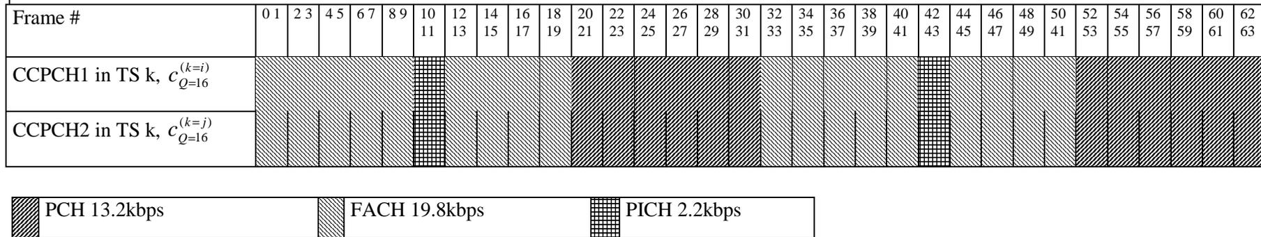
Figure CAF.2: Example for a multiframe structure for S-CCPCHs and PICH that is repeated every 64th frame,  $i, j=1 \dots 16$  ( $i \neq j$ ),  $k \neq 0, 1$ , (128 sub-frame)
