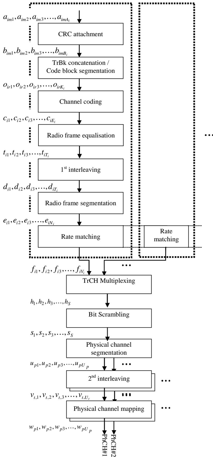
Figure 1A2: Transport channel multiplexing structure for uplink and downlink of 1.28Mcps TDD
