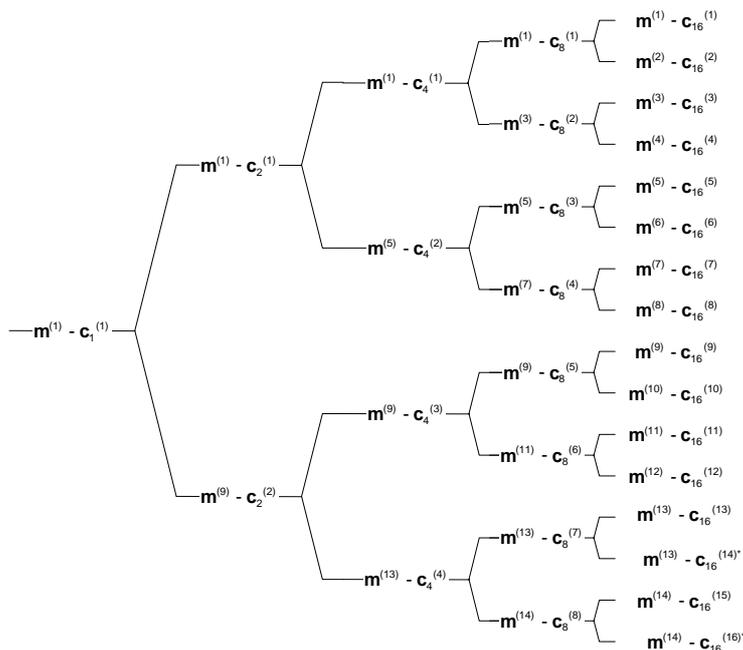
Figure AA.2B.2.2: Association of Midambles to Spreading Codes for K=14
