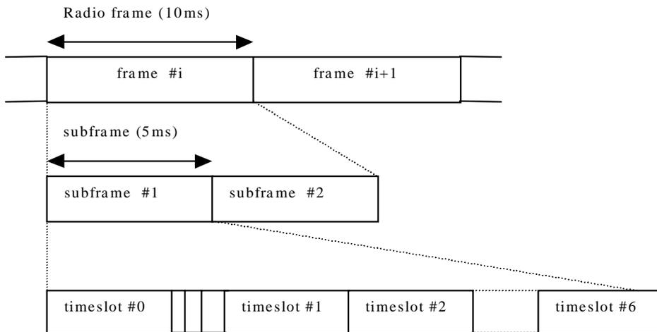
Figure 4918A: Physical channel signal format for 1.28Mcps TDD option
