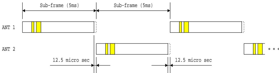
Figure 7: Example for the antenna switching pattern for TSTD transmission of DPCH/PDSCH and P-CCPCH: all physical channels are transmitted with TSTD and are using the same antenna in the sub-frame.
