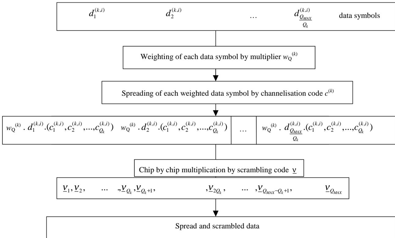
Figure 2: Spreading of data symbols
