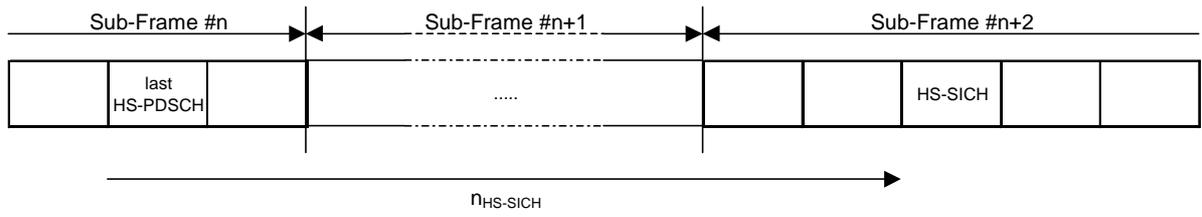
Figure 25.38: Timing for HS-DSCH and HS-SICH for different radio frame configurations for a given UE
