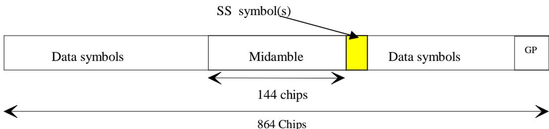
**Figure 4.618H: Position of ULSC information in the traffic burst (downlink and uplink)**
