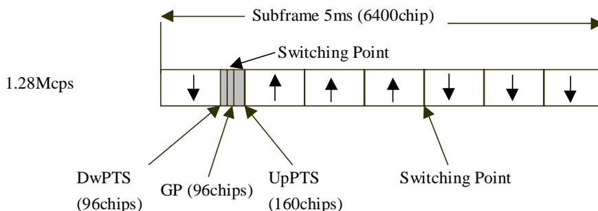
**Figure 2018B: Structure of the sub-frame for 1.28Mcps TDD option**
