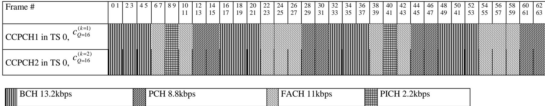
Figure CAF.1: Example for a multiframe structure for CCPCHs and PICH that is repeated every 64th frame (128 sub-frame)
