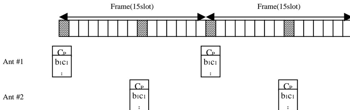
Figure 3: Antenna Switching Pattern (Case 2)
