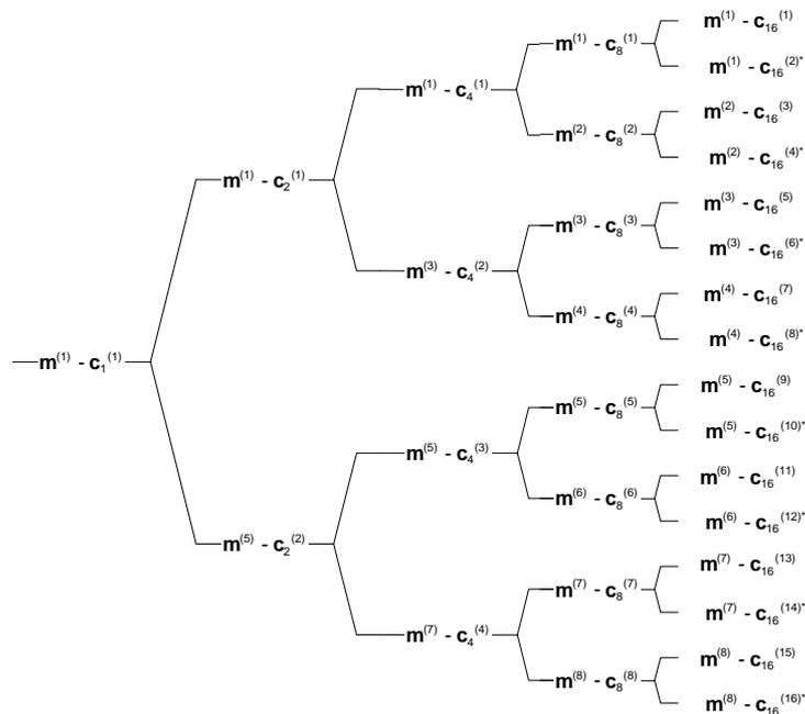
Figure AA.5B.2.5: Association of Midambles to Spreading Codes for K=8
