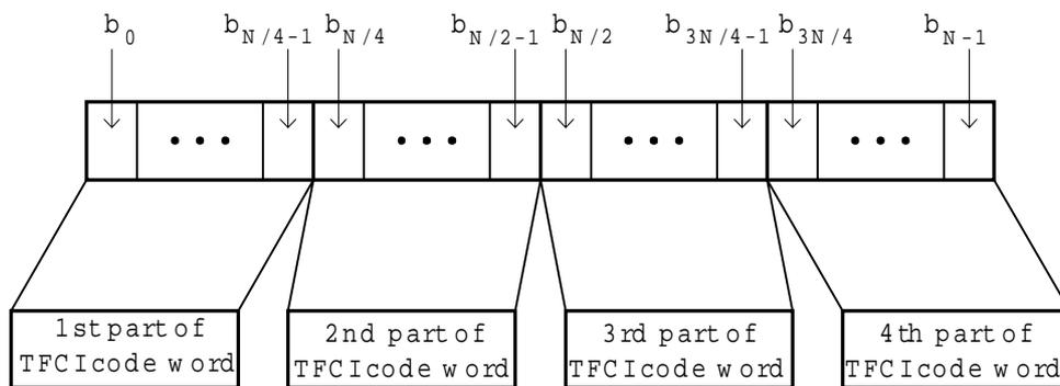
**Figure 940: Mapping of TFCI code word bits to TFCI position in 1.28 Mcps TDD option, where  $N = N_{\text{TFCI code word}}$**
