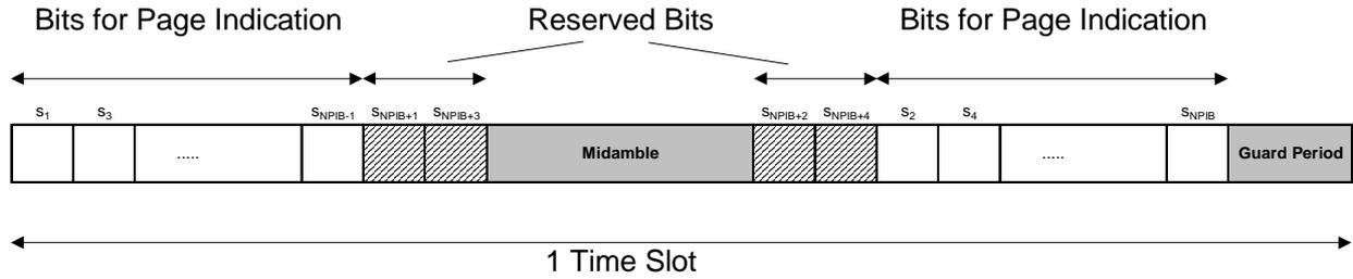
**Figure 15: Transmission and numbering of paging indicator carrying bits in a PICH burst**
