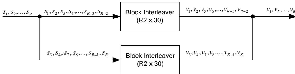
Figure 18.18b: Interleaver structure for HS-DSCH with 16-QAM modulation
