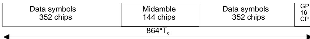
Figure 2218D: Burst structure of the traffic burst format (GP denotes the guard period and CP the chip periods)
