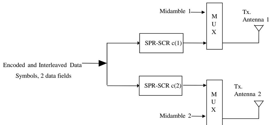
Figure 4: Block Diagram of the transmitter SCTD
