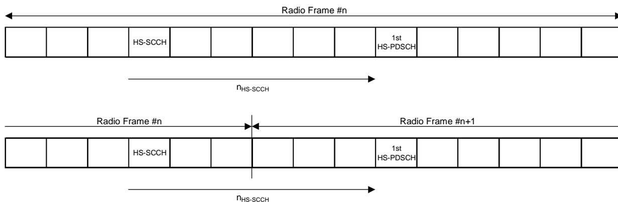
Figure 21A33: Timing for HS-SCCH and HS-DSCH for different radio frame configurations for a given UE
