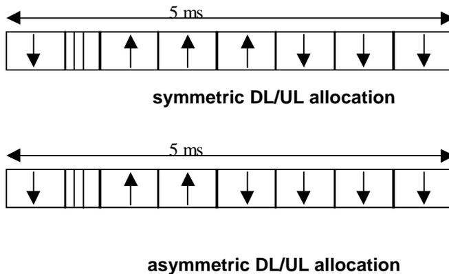
Figure 18C24: 1.28Mcps TDD sub-frame structure examples
