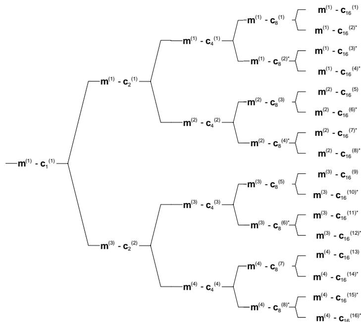
Figure AA.7B.2.7: Association of Midambles to Spreading Codes for K=4
