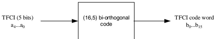
**Figure 78: Channel coding of short length TFCI bits**
