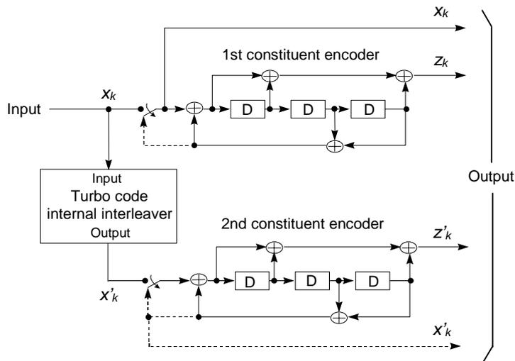
**Figure 34: Structure of rate 1/3 Turbo coder (dotted lines apply for trellis termination only)**
