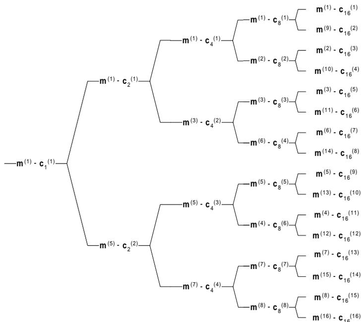
Figure A-1A.1: Association of Midambles to Spreading Codes for Burst Type 1/3 and  $K_{Cell}=16$
