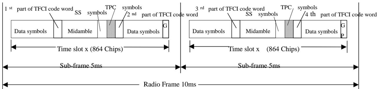
Figure 18F24: Position of the TFCI code word in the traffic burst in case of TPC and SS in 1.28 Mcps TDD
