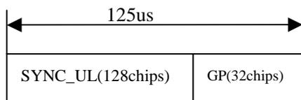
**Figure [2818J](#): burst structure of the UpPCH ( UpPTS)**
