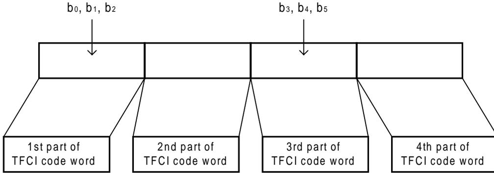
Figure 1415: Mapping of TFCI code word bits to timeslot in 1.28 Mcps TDD option when  $N_{\text{TFCI code word}} = 6$
