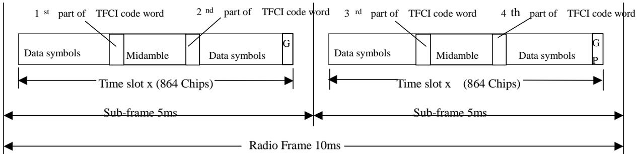
Figure 18E23: Position of the TFCI code word in the traffic burst in case of no TPC and SS in 1.28 Mcps TDD
