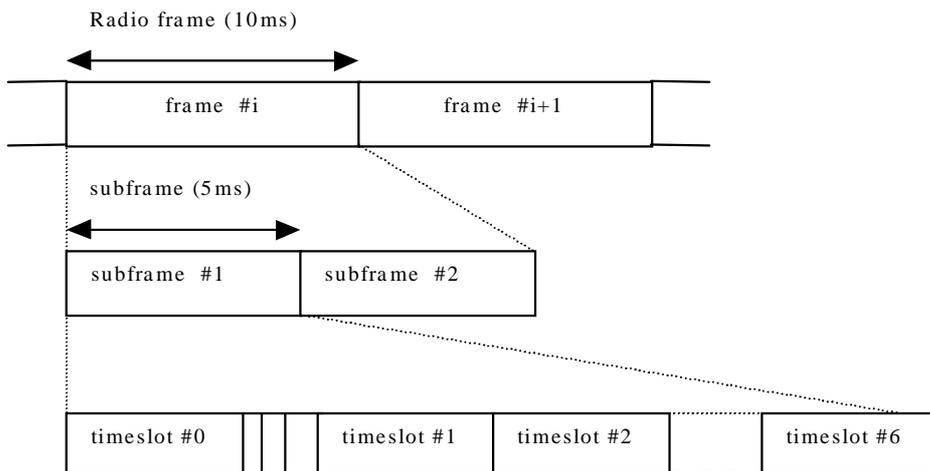
**Figure 18A49: Physical channel signal format for 1.28Mcps TDD option**
