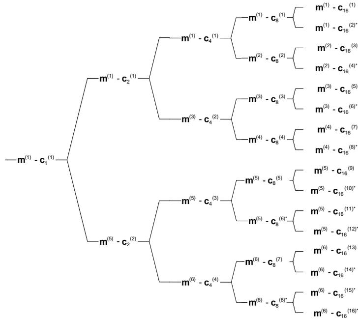
Figure AAB.2.6: Association of Midambles to Spreading Codes for K=6
