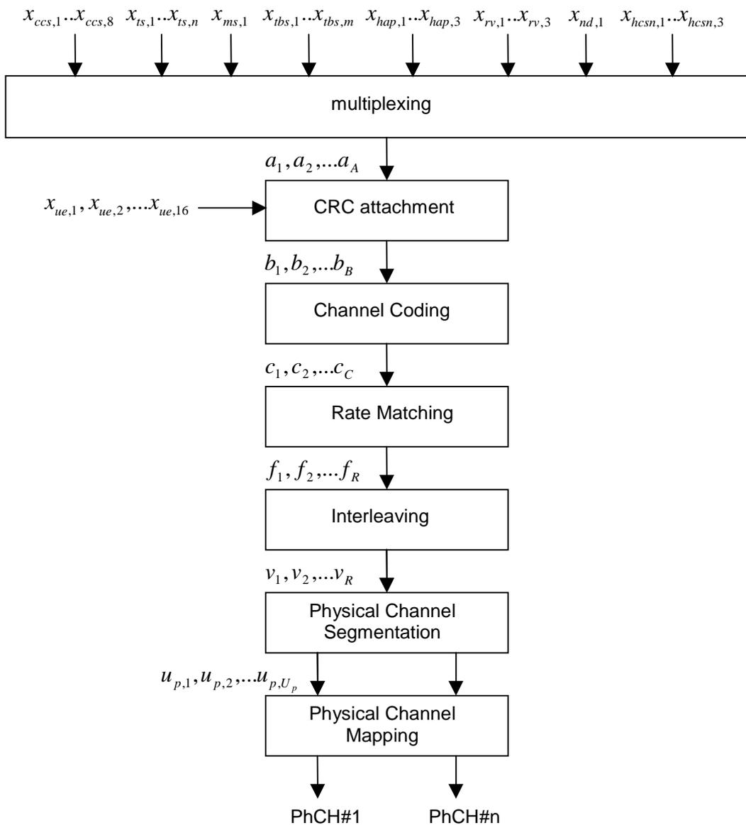
Figure 4.6.19 Coding and Multiplexing for HS-SCCH
