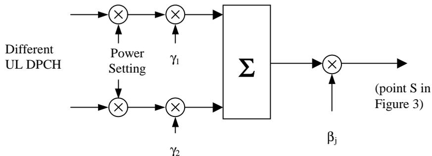
**Figure 4: Combination of different physical channels in uplink**
