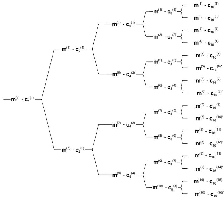
Figure AA.4B.2.4: Association of Midambles to Spreading Codes for K=10
