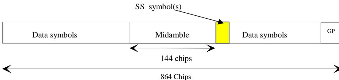
**Figure 18H26: Position of ULSC information in the traffic burst (downlink and uplink)**
