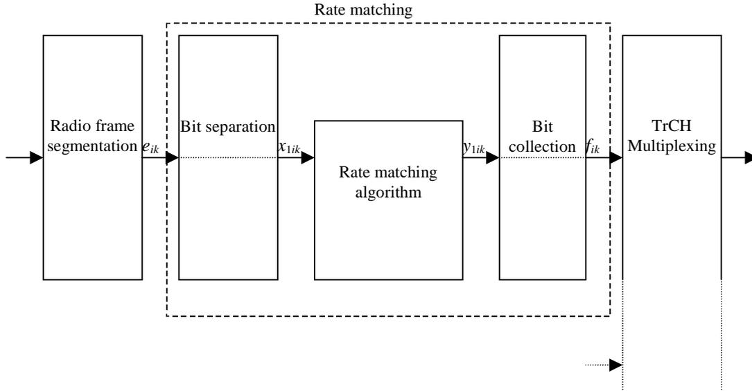
**Figure 56: Rate matching for uncoded TrCHs, convolutionally encoded TrCHs, and for turbo encoded TrCHs with repetition**
