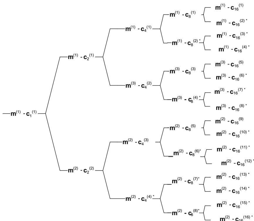
Figure A-5A.5: Association of Midambles to Spreading Codes for Burst Type 2 and  $K_{Cell}=3$
