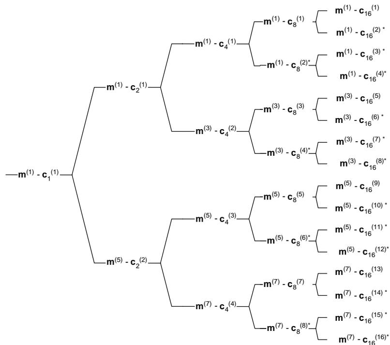
Figure A.3-3: Association of Midambles to Spreading Codes for Burst Type 1/3 and  $K_{Cell}=4$
