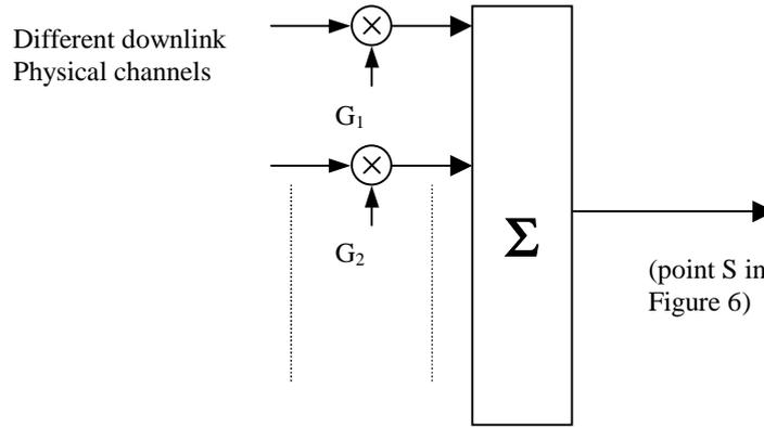
**Figure 7: Combination of different physical channels in downlink**
