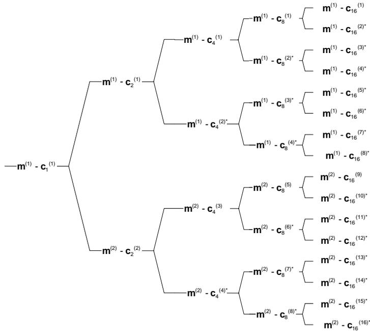
Figure AAB.2.8: Association of Midambles to Spreading Codes for K=2
