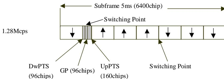
**Figure 18B20: Structure of the sub-frame for 1.28Mcps TDD option**
