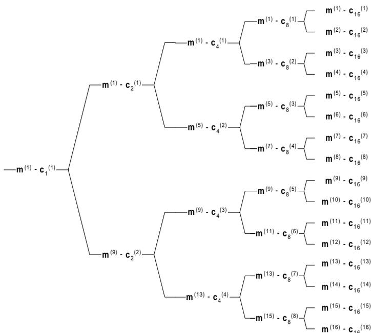
Figure AAB.2.1: Association of Midambles to Spreading Codes for K=16
