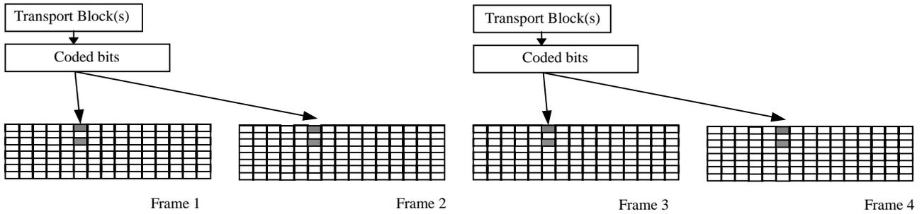
**Figure 2034: Mapping of Transport Blocks onto the physical bearer**
