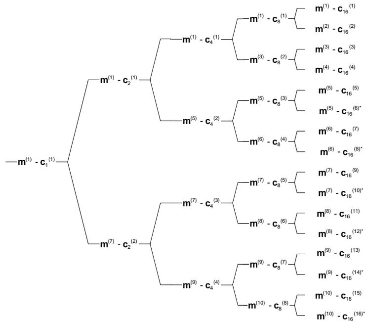
Figure AAB.2.4: Association of Midambles to Spreading Codes for K=10
