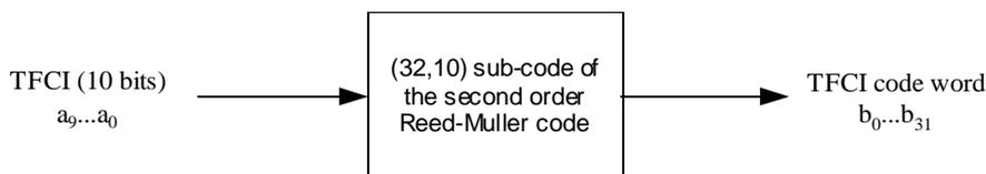
**Figure 67: Channel coding of the TFCI bits**
