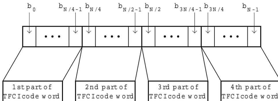
**Figure 1344: Mapping of TFCI code word bits to timeslot in 1.28 Mcps TDD option, where  $N = N_{\text{TFCI code word}}$**
