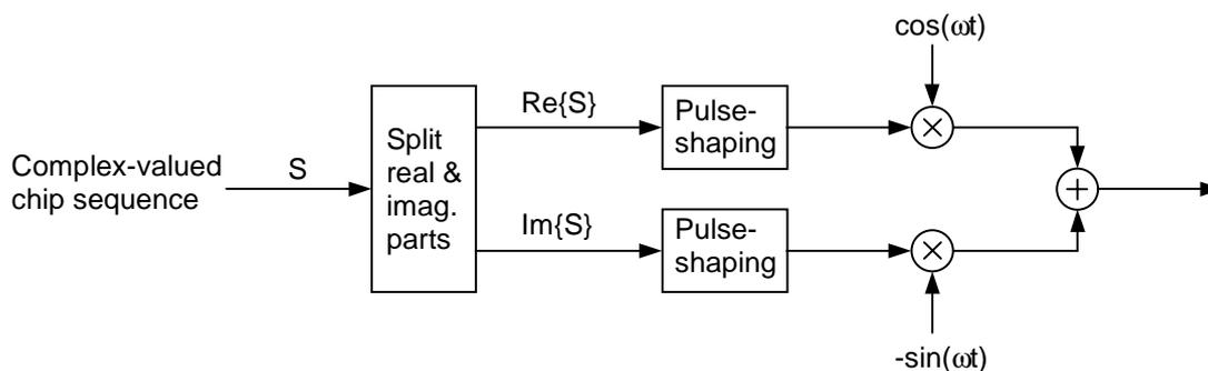
Figure 6: Modulation of complex valued chip sequences
