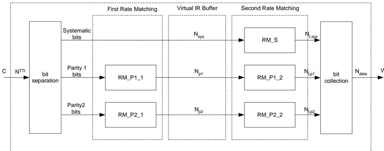
Figure 1647: HS-DSCH hybrid ARQ functionality
