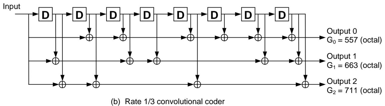
**Figure 23: Rate 1/2 and rate 1/3 convolutional coders**
