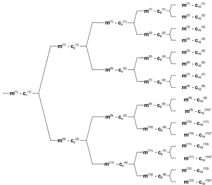
Figure AAB.2.3: Association of Midambles to Spreading Codes for K=12
