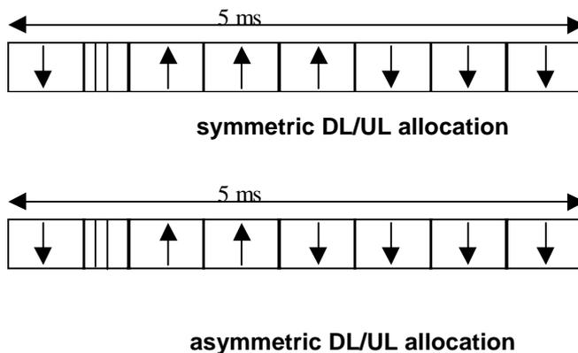
Figure 2418C: 1.28Mcps TDD sub-frame structure examples
