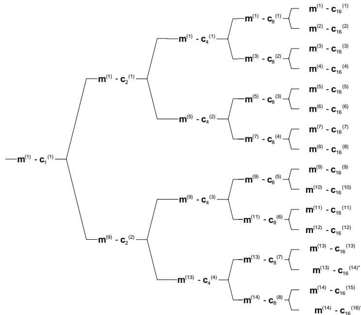
Figure AAB.2.2: Association of Midambles to Spreading Codes for K=14
