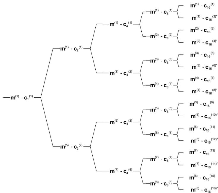
Figure AAB.2.5: Association of Midambles to Spreading Codes for K=8
