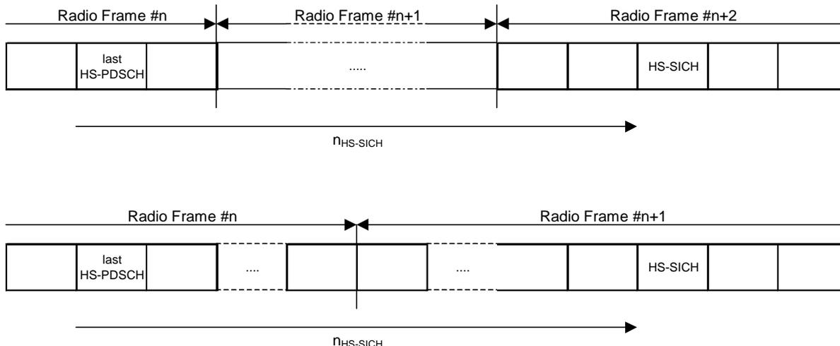
Figure 21B34: Timing for HS-DSCH and HS-SICH for different radio frame configurations for a given UE
