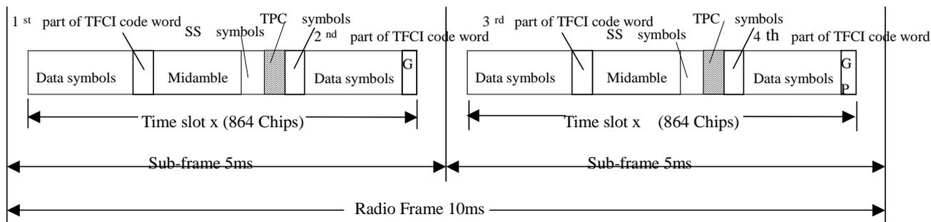
**Figure 24.18F: Position of the TFCI code word in the traffic burst in case of TPC and SS in 1.28 Mcps TDD**
