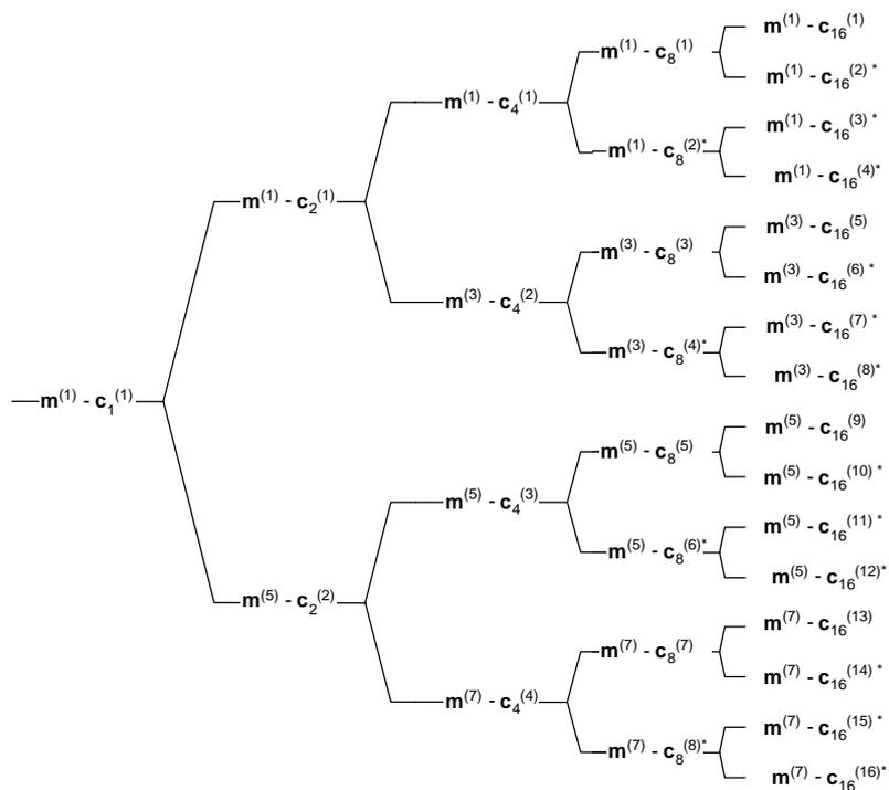
Figure A-3A.3: Association of Midambles to Spreading Codes for Burst Type 1/3 and  $K_{Cell}=4$
