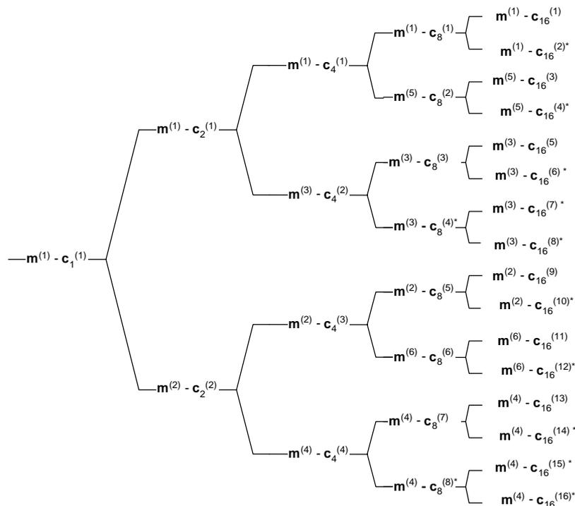
Figure A-4A.4: Association of Midambles to Spreading Codes for Burst Type 2 and  $K_{Cell}=6$
