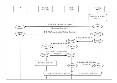
**Soft Handover - Radio Link Deletion (Branch Deletion)**
