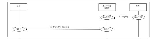
Paging for a UE in RRC Connected Mode when the UTRAN coordinates the paging request with the existing RRC connection using DCCH
