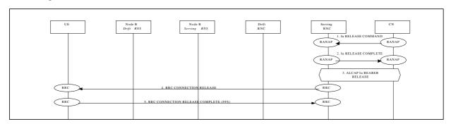
RRC Connection release of a common channel
