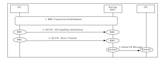
**NAS Signalling Connection Establishment**
