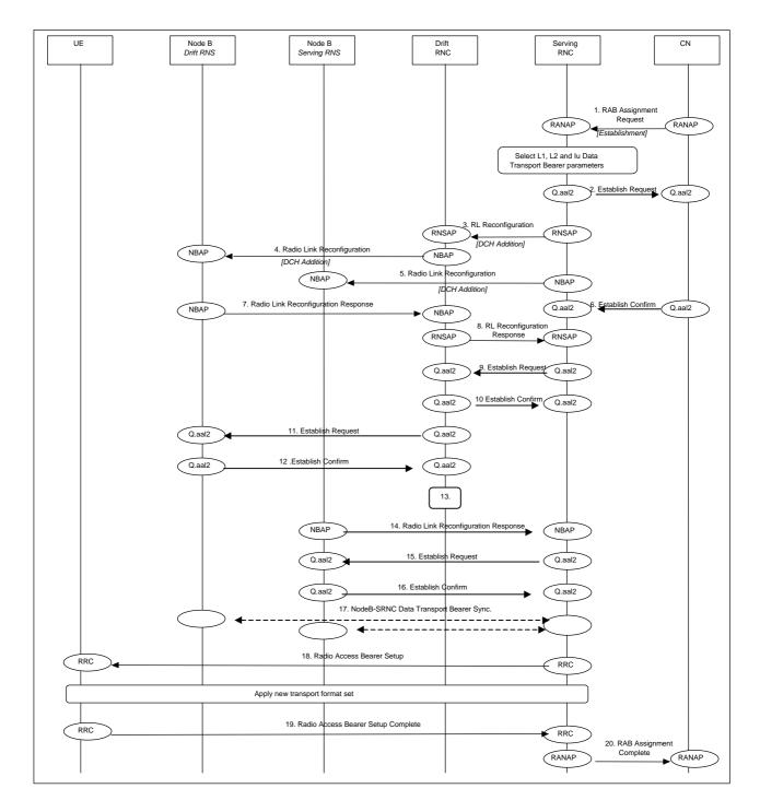
Radio Access Bearer Establishment - DCH - DCH Establishment - Unsynchronised
