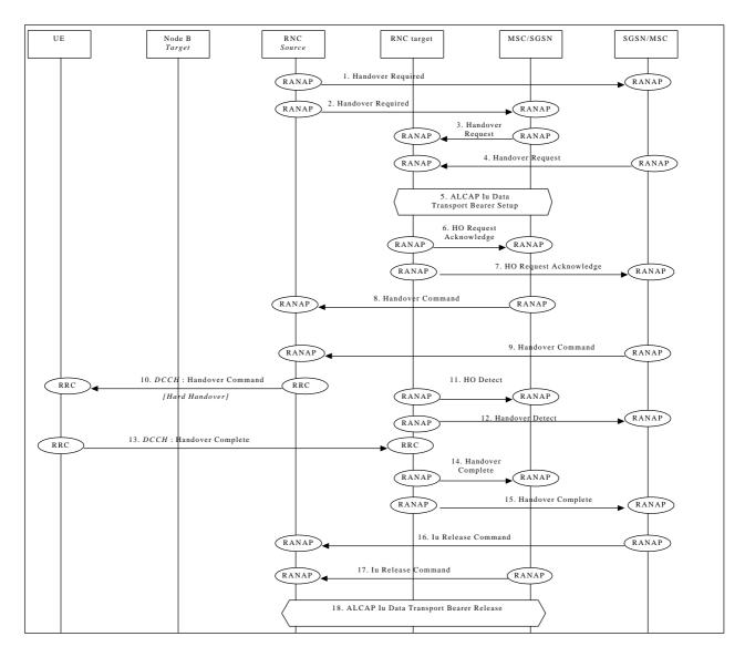
Inter-RNS Hard Handover with switching in the CN (UE connected to two CN nodes)
