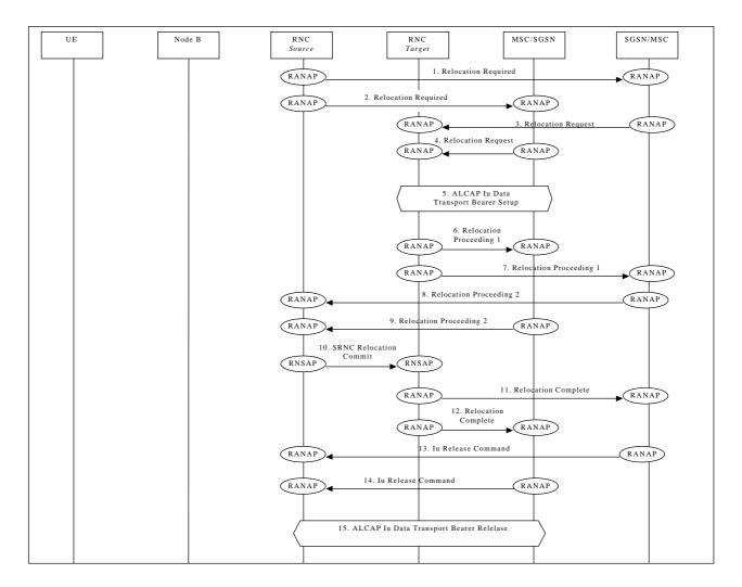
SRNC Relocation (UE connected to two CN nodes)
