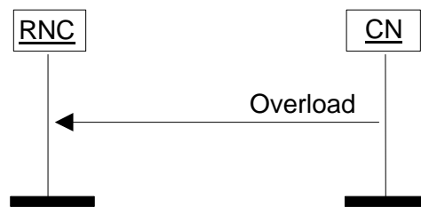
Figure 8. Overload at the CN.
