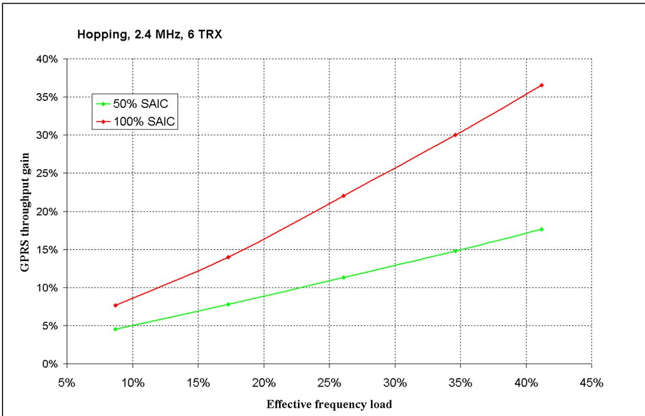
**Figure 2. Relative GPRS throughput gain versus load with two different SAIC proportions.**
