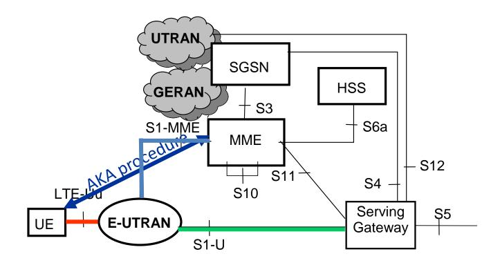
Confidentiality and integrity for signalling and confidentiality for user plane (RRC & NAS)
