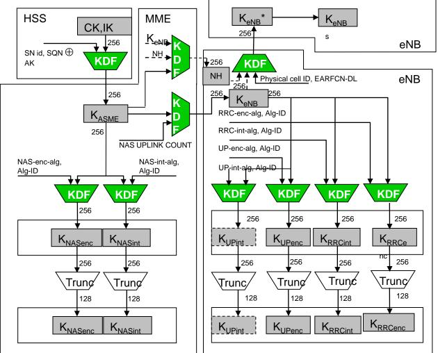
Key distribution and key derivation scheme for EPS (network side), found in 33.401 Key Derivation Function (KDF) specification can be found in 33.220
